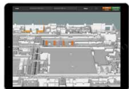
Inspection with BIM data and Model Viewer on mobile device Image courtesy of SUNeVision Holdings Limited
