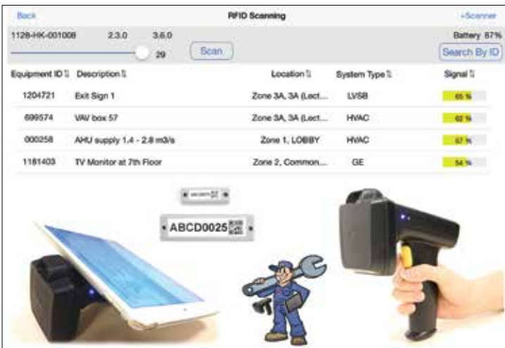
The screen capture showing the results of RFID scanning at mobile terminal for further enquiry of asset information Image courtesy of Electrical and Mechanical Services Department, HKSAR Government
