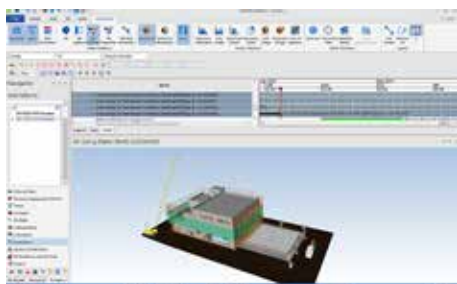
4D method statement to demonstrate construction activities of the Membrane Facilities Building and Membrane Tanks Image courtesy of Drainage Services Department, HKSAR Government and Summit Technology (Hong Kong) Limited
