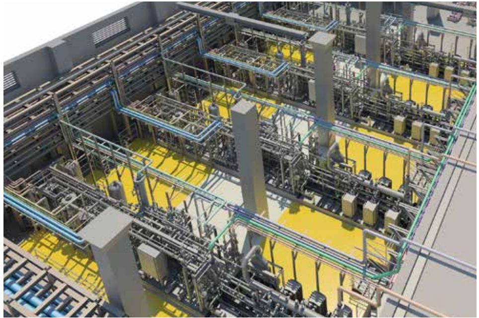
BIM Facilitated Interdisciplinary Coordination involving Mechanical and Electrical Equipment, Piping, Utilities for Building Services, Civil and Structural Design Image courtesy of Water Supplies Department, HKSAR Government
