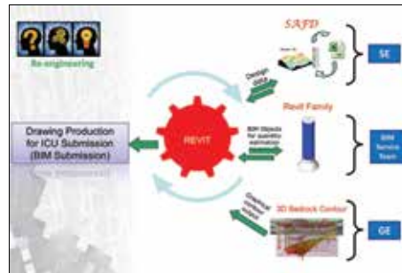
FIGURE 3 - Workflow of BIM-SAFD for BIM Submission Image courtesy of Hong Kong Housing Authority, HKSAR Government
