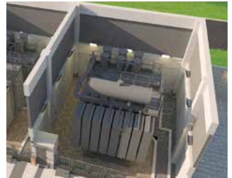
Virtual model of the high voltage transformer bay facilitates the planning for future operation and maintenance activities Image courtesy of CLP Power Hong Kong Limited
