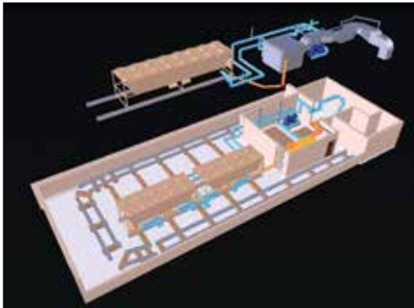
Visualisation of the construction sequence: Phase 1 – Demolition of existing chiller, pipeworks and ductworks Image courtesy of Arup and Greenwich Investors Limited
