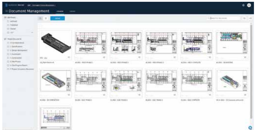
BIM 360 as a common data environment Image courtesy of Arup and Greenwich Investors Limited
