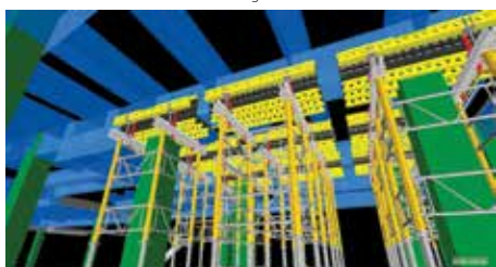
Falseworks for buildings to eliminate major system conflicts, control site safety and cost control Image courtesy of Civil Engineering and Development Department, HKSAR Government and AECOM Asia Company Limited and Leighton-China State Joint Venture
