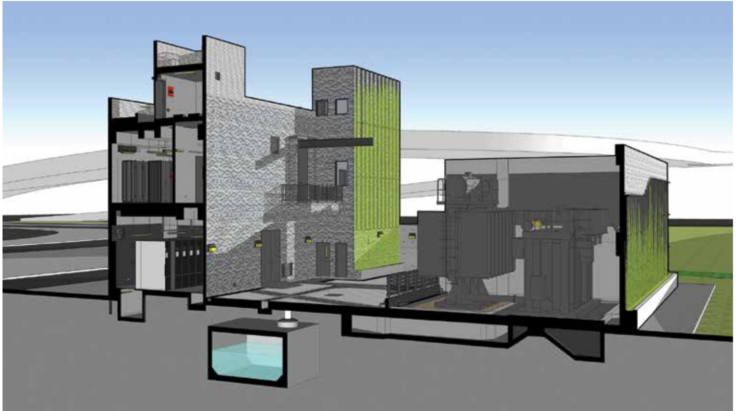
BIM Model provides an accurate sense of presence of building structure that is yet to be built. Improvement to the design can be identified easily prior to the construction Image courtesy of CLP Power Hong Kong Limited
