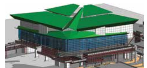
Temporary Works Design with Scaffolding Image courtesy of Hip Hing Construction Company Limited
