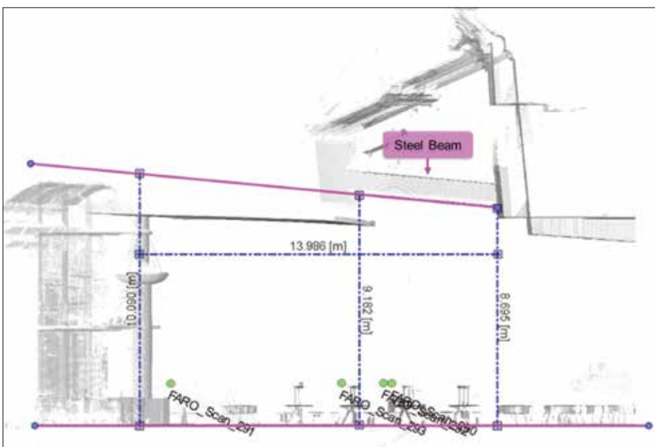
Existing Structure Verification via 3D Laser Scanning Image courtesy of Hip Hing Construction Company Limited
