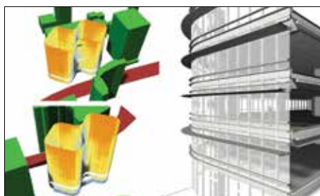
Solar heat gain analysis with building envelope from BIM model was carried out to optimize shading fins design Image courtesy of Link Real Estate Investment Trust and Nan Fung Development Limited
