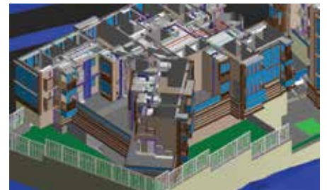
Project BIM models showing Coordinated building services Image courtesy of Nan Fung Development Limited
