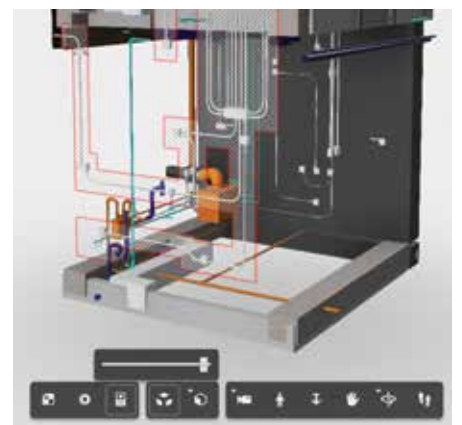
3D view of 'No nail zone' BIM models on web-based viewer Image courtesy of Nan Fung Development Limited
