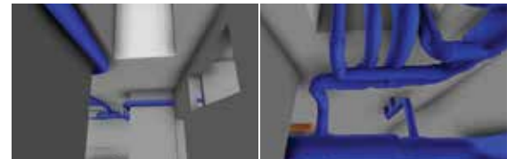
Laser scanning technology was deployed on site to obtain accurate as-built models Image courtesy of Nan Fung Development Limited
