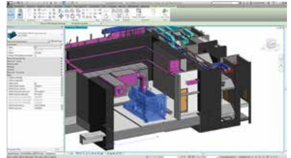
Equipment and asset information embedded in project BIM model for future Facility Management Image courtesy of Nan Fung Development Limited
