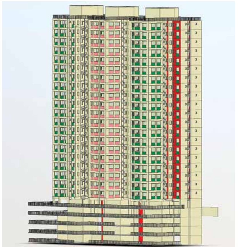
With BIM technology, 3D model can be created from existing drawings as a better way of visualization Image courtesy of Urban Renewal Authority
