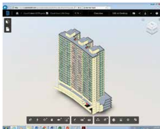
With BIM technology, 3D model can be created from existing drawings as a better way of visualization Image courtesy of Urban Renewal Authority
