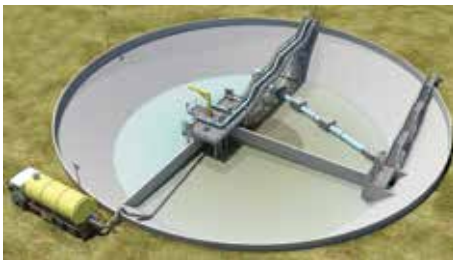
Periodic Removal of Sludge Accumulated in the Temporary Washwater Recovery Tank Image courtesy of Water Supplies Department, HKSAR Government and Ming Hing – Ming Hing Civil – Vasteam Joint Venture and Summit Technology (Hong Kong) Limited
