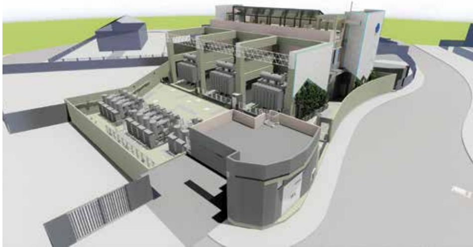
BIM model provides an accurate sense of presence of building structure that is yet to be built. Improvement to the design can be identified easily prior to the construction. Image Courtesy of CLP Power Hong Kong Limited
