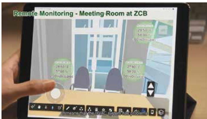
Integration of BIM-AM System and IoT Technology for remote monitoring Image courtesy of Electrical and Mechanical Services Department, HKSAR Government
