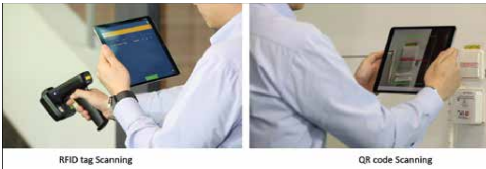
Asset fast located by QR code / RFID tag scanning Image courtesy of Electrical and Mechanical Services Department, HKSAR Government
