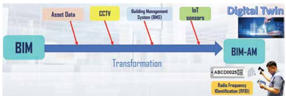
Transformation from BIM to BIM-AM Image courtesy of Electrical and Mechanical Services Department, HKSAR Government
