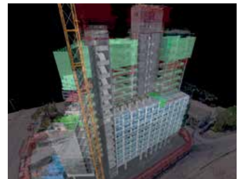
3D Drone Scanning Result Incorporated with 4D Simulation Image Courtesy of Hip Hing Engineering Company Limited and Hong Kong Science and Technology Parks Corporation and Leigh & Orange Limited
