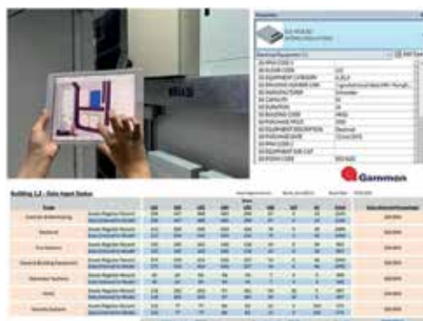
Digital asset data storage in BIM. Image Courtesy of Global Switch
