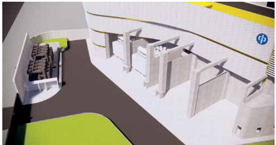
BIM enhances the multidisciplinary design collaboration and optimisation for high voltage plant equipment installation. Image Courtesy of CLP Power Hong Kong Limited
