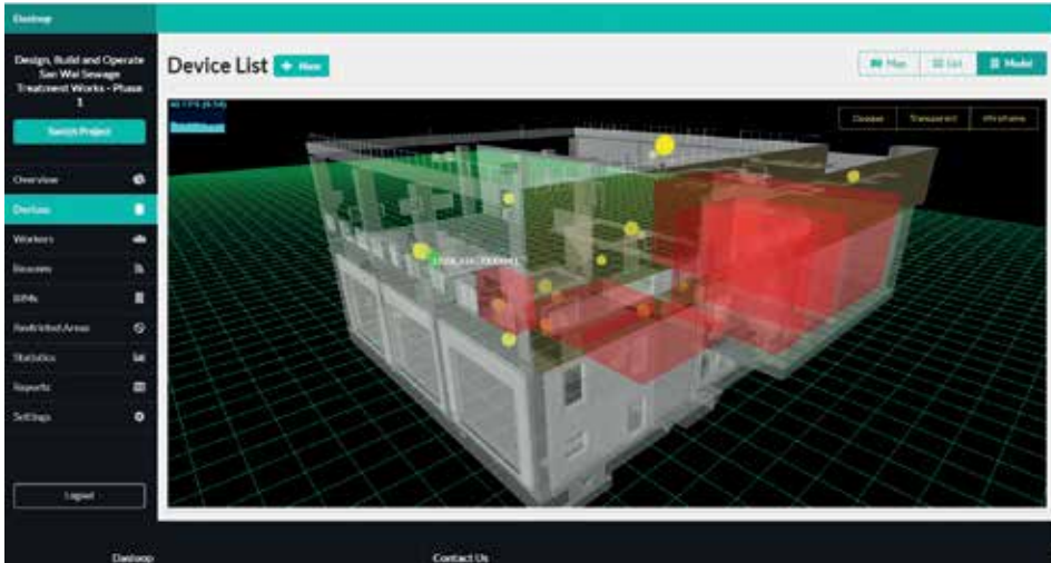
IoT Smart Safety Helmet Integrated with BIM Image Courtesy of Drainage Services Department, HKSAR Government and AECOM Asia Company Limited and ATAL-Degremont-China Harbour Joint Venture
