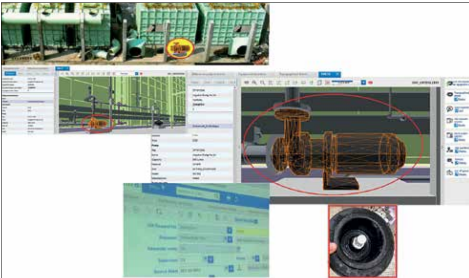
BIM Viewer on Computerised Maintenance Management System Image Courtesy of Drainage Services Department, HKSAR Government and AECOM Asia Company Limited and ATAL-Degremont-China Harbour Joint Venture
