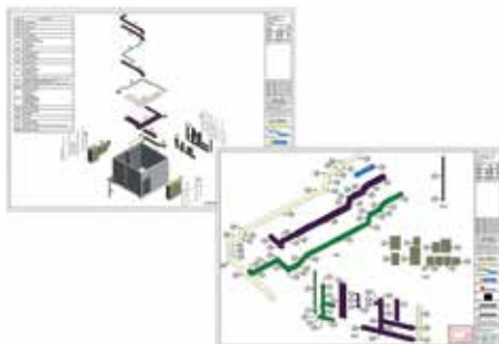
DfMA plant room designed by BIM for manufacture. Image Courtesy of Global Switch
