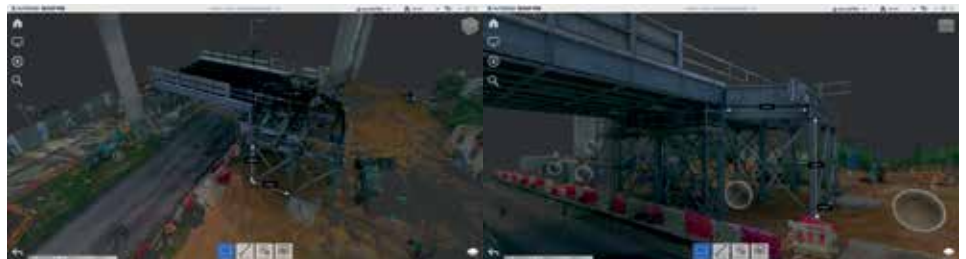
Survey check and measurement using Autodesk® Recap Pro Image Courtesy of Drainage Services Department, HKSAR Government and AECOM Asia Company Limited
