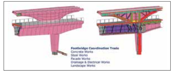
Use of parametric model for complex forms such as sculptural footbridge column made it possible for project team to respond to design changes and model update after inter-disciplinary coordination more rapidly. Image Courtesy of Nan Fung Development Limited
