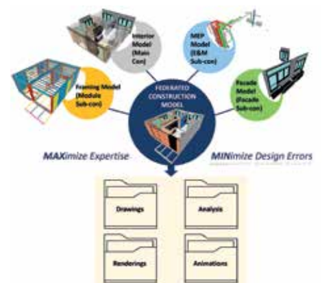
BIM Collaboration Strategy of MiC Modules Design Image Courtesy of Hip Hing Engineering Company Limited and Hong Kong Science and Technology Parks Corporation and Leigh & Orange Limited
