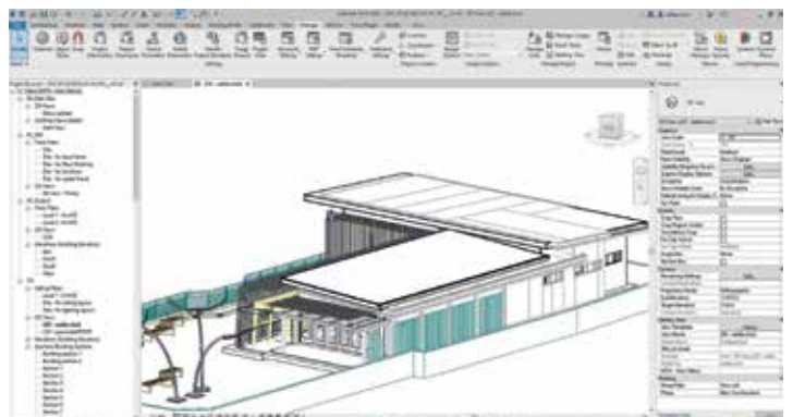
Revit Model of Community Liaison Centre Image Courtesy of Drainage Services Department, HKSAR Government and AECOM Asia Company Limited and China State Construction Engineering (Hong Kong) Limited and MTECH Engineering Company Limited
