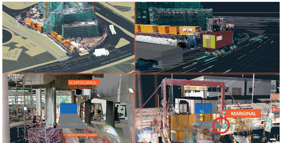
Swept Path Simulation of Module-Loading Vehicle Along the Site Image Courtesy of Hip Hing Engineering Company Limited and Hong Kong Science and Technology Parks Corporation and Leigh & Orange Limited
