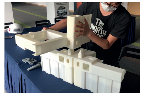
Demonstration of MiC Module Connection Using 3D Printed Components Image Courtesy of Hip Hing Engineering Company Limited and Hong Kong Science and Technology Parks Corporation and Leigh & Orange Limited
