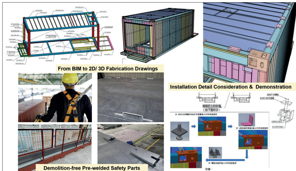
Design for Demolition-Free Pre-Welded Safety Parts in Permanent Module Frame Image Courtesy of Hip Hing Engineering Company Limited and Hong Kong Science and Technology Parks Corporation and Leigh & Orange Limited
