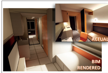
BIM-Rendered Co-Living Unit for Pre-Mockup Visualization Image Courtesy of Hip Hing Engineering Company Limited and Hong Kong Science and Technology Parks Corporation and Leigh & Orange Limited
