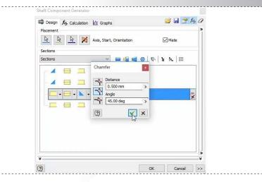
Define a 'Chamfer' for the second edge of the section, using the values shown.
