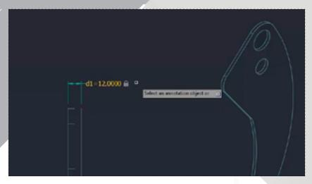
Edit the d1 dimension, defining the part's thickness, to 12mm. Save the AutoCAD file, and then go back to the Inventor assembly file.
