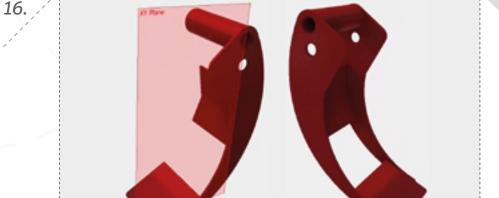
Mirror the part about the XY Plane to complete the Gripper Arm assembly design.
