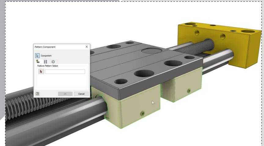
Reopen the 'Pattern Component' command from the marking menu. Select the two linear guide subassemblies as the components to be patterned.
