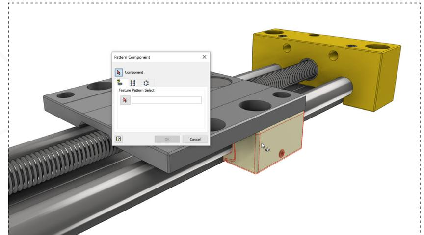
Right click to open the marking menu and select 'Pattern Component.' Select the linear guide subassembly as the component to be patterned.
