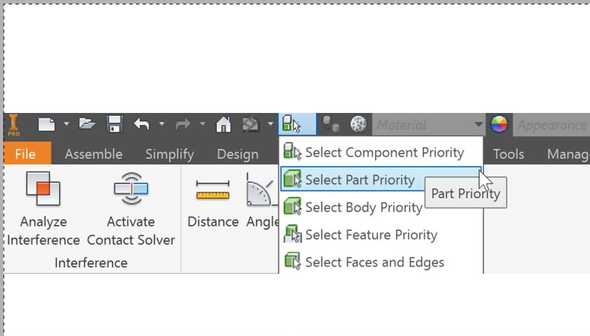
Continue with the assembly from Part 2. Make sure 'Select Part Priority' is selected. In the ribbon, select the 'Inspect' tab and open 'Analyze Interference'.
