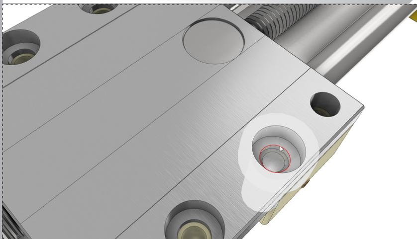
Select the circular edge as shown to define the placement of the bolt. The bolt will autosize based on the dimensions of the hole.
