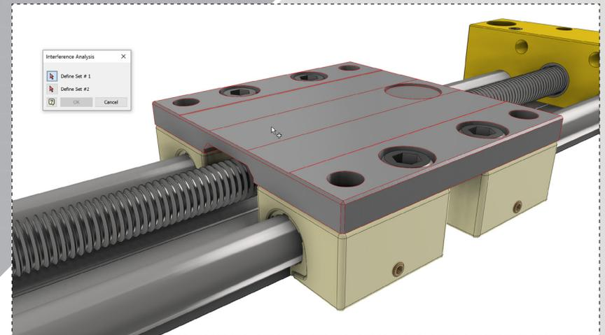
The objective is to determine if there is any interference between the top plate and the linear guides placed and patterned in Part 1. For Set #1, select the plate as shown.
