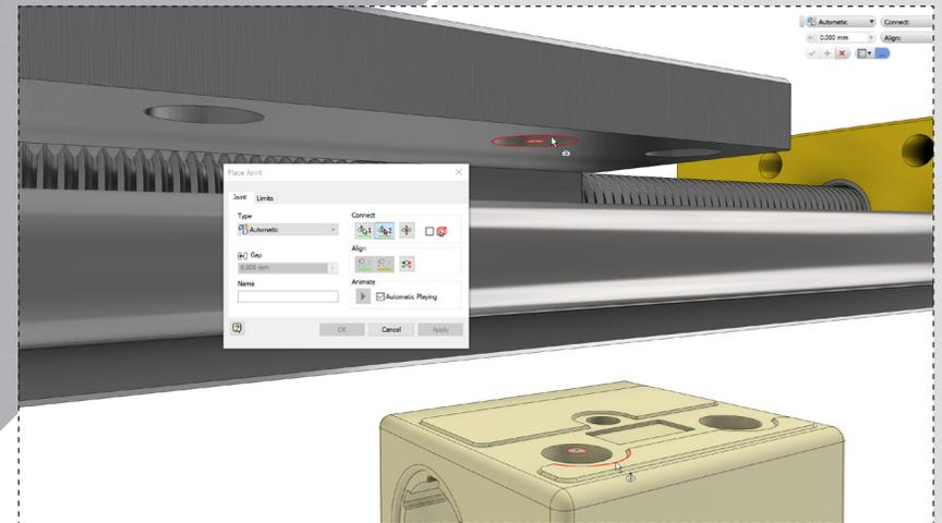
Open the marking menu and select 'Joint.' Click the circular features as shown and then select 'Apply' to create a rotational joint.
