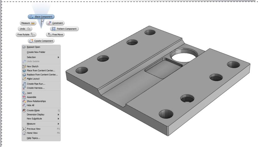
In the model window, right click to bring up the marking menu. Select 'Place Component' and choose **SWZ-W-104003.ipt**. Left click anywhere in the model window to place and then hit 'ESC'.
