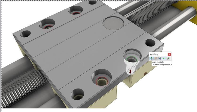
Make sure the AutoDrop option is selected and click the green check mark to place bolts in all four holes simultaneously.
