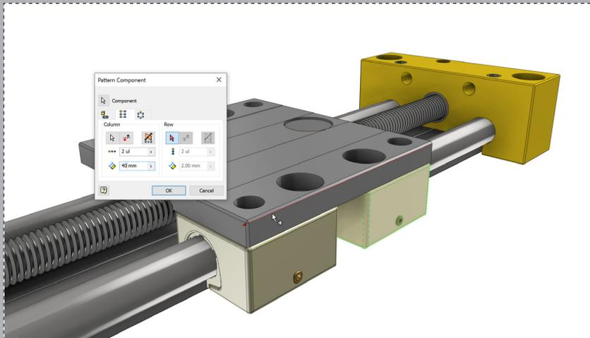
Pick the rectangular pattern tab. In the 'Column' section, click the cursor icon and select the edge of the assembly shown (flip if needed). Change the spacing to 40mm and click 'OK'.
