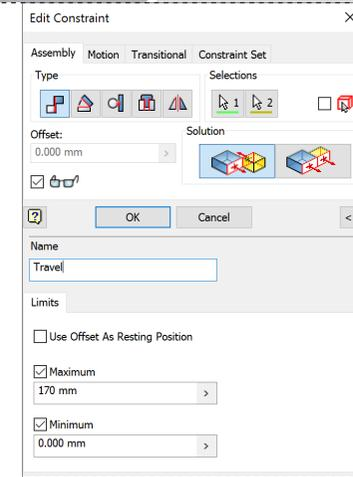
Click the double arrow (>>) in the bottom right corner. Click the check marks next to 'Maximum' and 'Minimum', entering 170mm in the 'Maximum' box and **Travel** in the 'Name' field.
