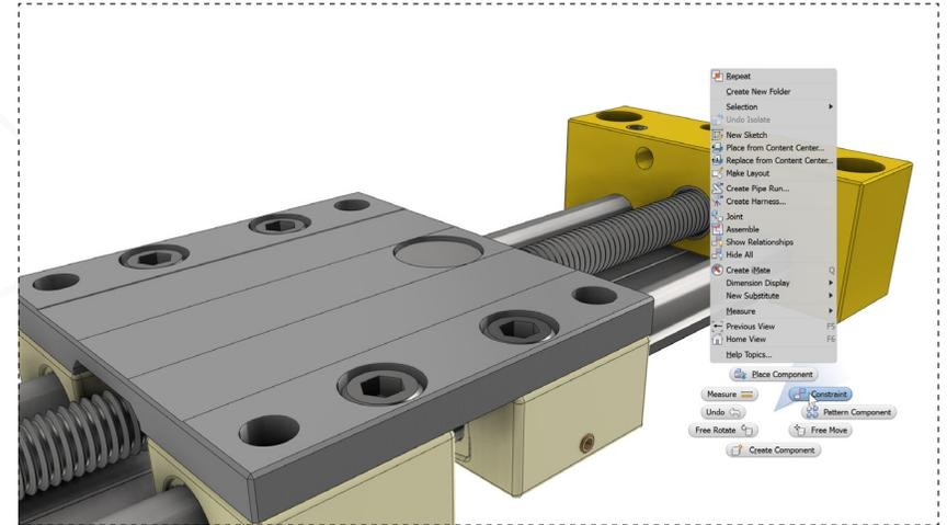
To setup the motion analysis, start the 'Constraint' command from the right click marking menu.
