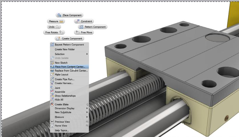
Continue with the assembly from Part 1. Right click to open the marking menu, and select 'Place from Content Center'.
