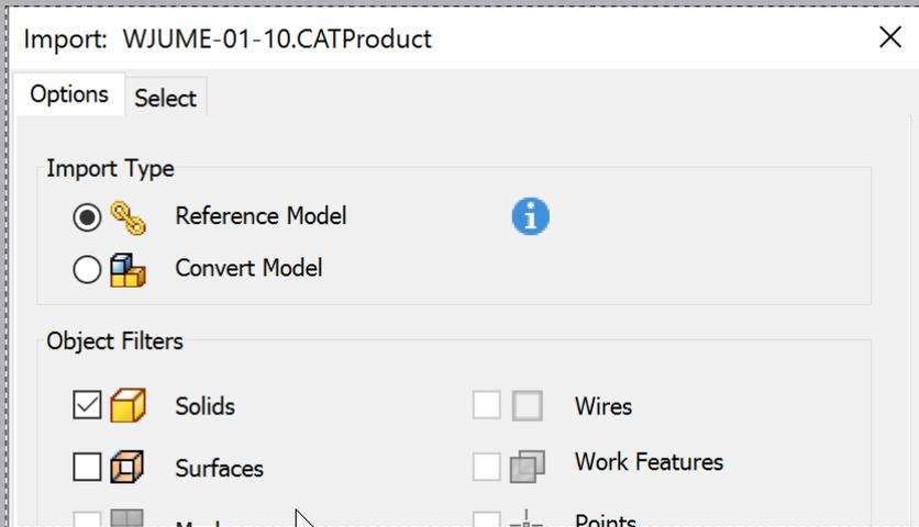
In the Import dialog, make sure Reference Model is selected and click 'OK.' Left click to place an instance of the model in the assembly and use 'ESC' to end the command.
