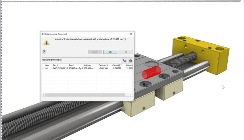
An interference is detected - between the nut and the threaded shaft. Inspect to make sure only the threaded area is in contact.
