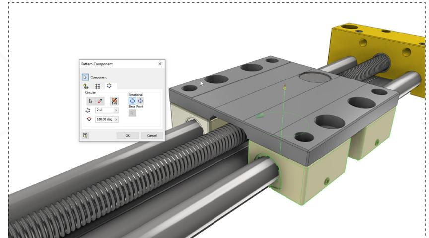
Change the number of instances to 2 and the angle to 180° and click 'OK' to complete the pattern. Save the assembly.
