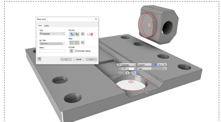
Right click to display the marking menu and choose 'Joint'. Select the two cylindrical surfaces shown to create the joint, flipping the orientation if necessary.
