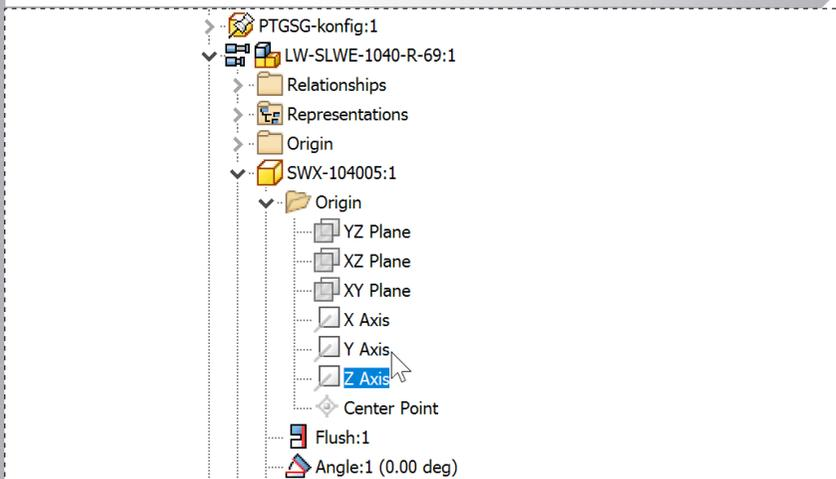
Pick the circular pattern tab. In the 'Circular' section, click the cursor icon. In the model tree, expand the tree as shown in the image above and select the Z-axis.
