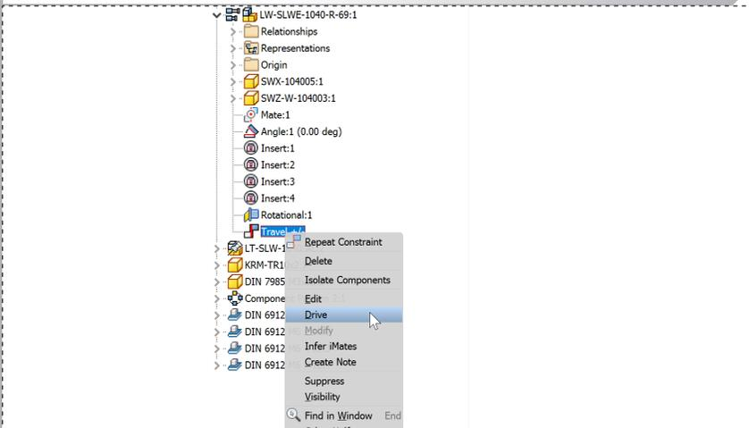
In the Model Tree, expand as shown and right click on the constraint named Travel. Select 'Drive'.
