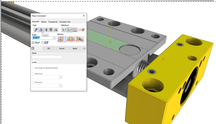
Change the 'Place Constraint' type to 'Angle' and select the two faces shown. Click 'OK' to apply and close the dialog.
