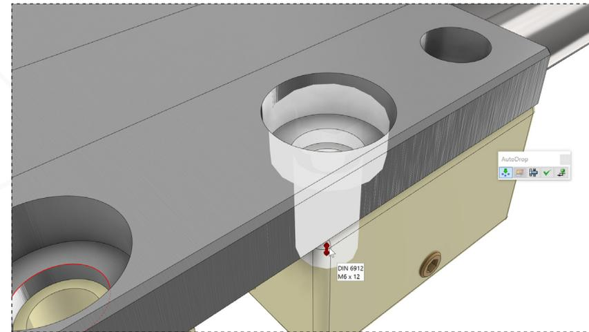
Adjust the height of the bolt by clicking and dragging the red arrow. The length should be 12mm (M6 x 12).
