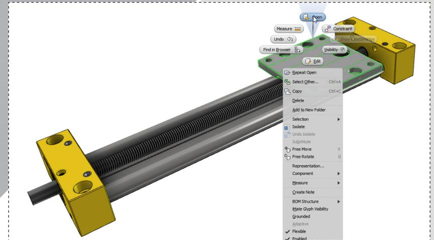
Select the sub-assembly **LW-SLWE-1040-R-69.iam** in the model window and right click to bring up the marking menu. Select 'open'.
