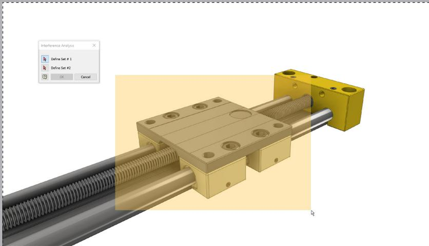
Restart the 'Analyze Interference' command. Window select the parts shown in the image above for Set #1.
