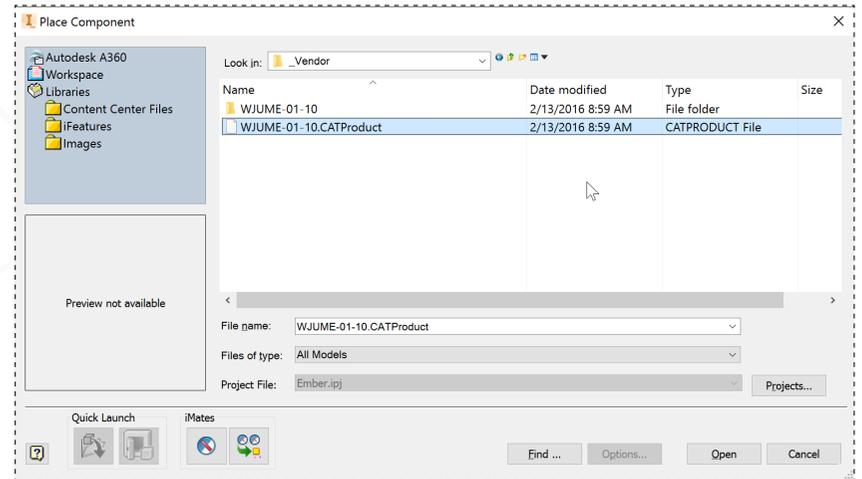
In the ribbon, open the drop down menu under the 'Place' icon and select 'Place Imported CAD File.' Navigate to the "\_Vendor" subfolder, and open **WJUME-01-10.CATProduct**.
