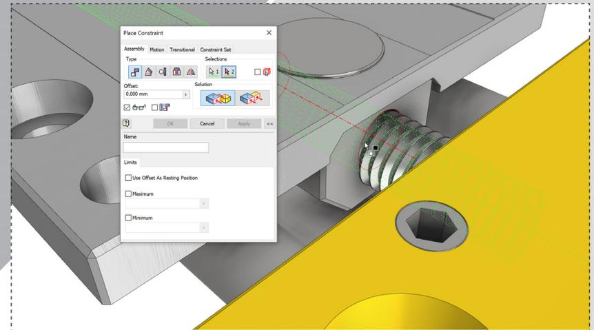
Open the marking menu and select 'Constraint'. Select the axes of the threaded rod and nut to place a mate constraint. Click 'Apply' in the dialog box to leave it open.
