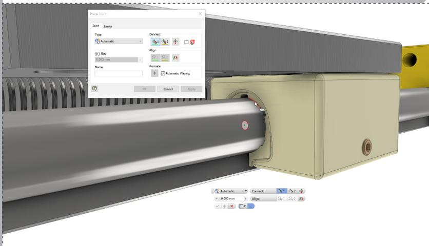
With the Joint dialog still open, click the circular edge of the bushing (as shown) and guide rail. Change the Joint Type to 'Cylindrical' in the dialog and flip if necessary. Click 'OK'.
