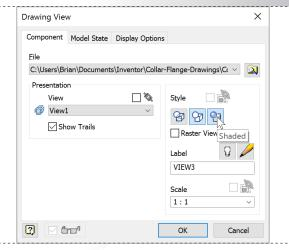
In the Style section of the dialog, make sure both 'Hidden Lines Removed' and 'Shaded' are selected and select 'OK'.
