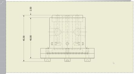
Start the 'General Dimension' command from the marking menu and add the dimensions as shown in the Front view.
