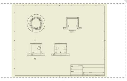
After breaking the alignment, move the view to the upper right quadrant of the drawing as shown.
