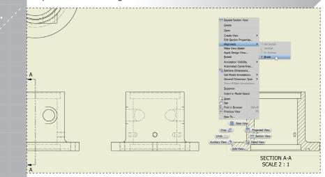
Break the forced alignment by right clicking on the view, selecting 'Alignment' and choosing 'Break'.
