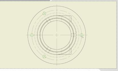
In the top view, select each of the four holes highlighted in green above. Select the hole you picked first a second time to complete the centerline. Right click and select 'Create'.
