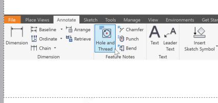
In the 'Annotate' tab inside the ribbon, select 'Hole and Thread'.
