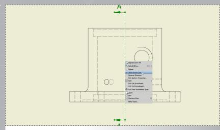
To remove the display of the selection line through the part in the Base view, right click the line and uncheck 'Show Entire Line'.
