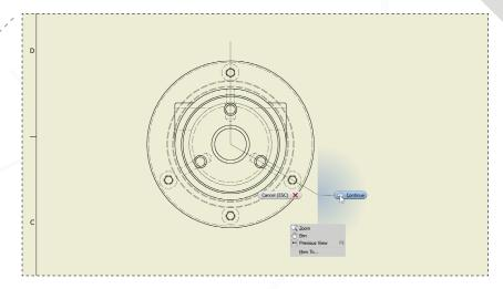
Right click inside the Top view and select 'Section View'. Draw the line as shown above to define the section, right click and select continue.
