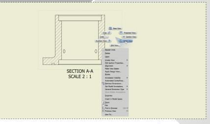
To create a detail view, right click inside the 'Section A-A' view and select 'Detail View' from the marking menu.
