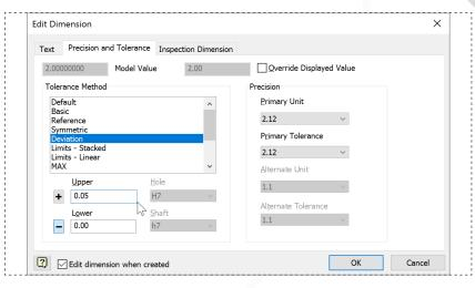
In the dialog box, open the 'Precision and Tolerance' tab. Select 'Deviation' as the method and enter 0.05 as the upper limit.
