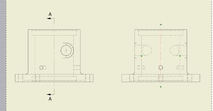
In the Base, Right, and Section A-A views, adjust the centerline length beyond the part by clicking the line and moving the green handle.
