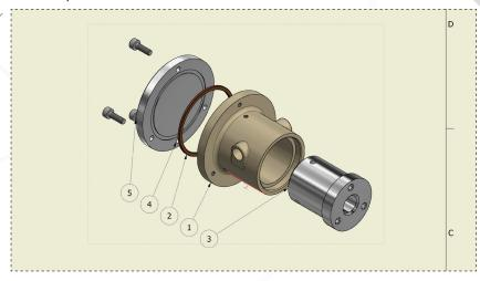
Select the edge of the flange highlighted in red as shown and then drag the balloons away from the part to their final placement to complete the drawing.
