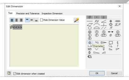
In the dialog box, add a 'Diameter' symbol at the beginning of the text field and select 'OK'. Right click in the model window and select 'OK' to finish the dimension command.
