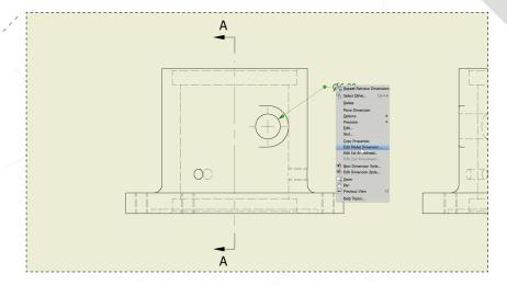
Right click on the 6mm diameter dimension and choose 'Edit Model Dimension' from the marking menu. With this, you can change 3D model parameters from within the drawing view.
