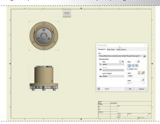
Open 'Base View' from the marking menu. Set the style to 'Hidden Line' and Scale to '2:1'. Click to place the view in the top left corner and then click below to create the side view.
