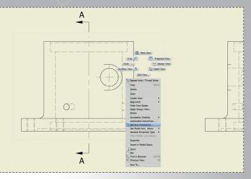
Inside the Base view, right click select 'Retrieve Dimensions' from the marking menu. This brings up all dimensions that were used to define the 3D model.
