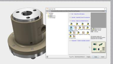
Reopen Collar-Flange-Assembly.iam. Create a new drawing by selecting 'New' from the ribbon menu and select the same drawing template as before, 'ANSI (mm).dwg'.
