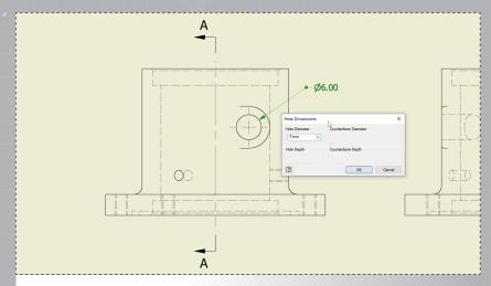
Change the Hole Diameter to 7mm and click 'OK'. The drawing will update immediately and the change will be carried over to the 3D model as well.
