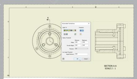
Place the view to the right. Right click inside Section A-A and select 'Automated Centerlines'. Select 'Cylindrical Features' in the dialog and check both boxes in 'Projection.' Click 'OK'.
