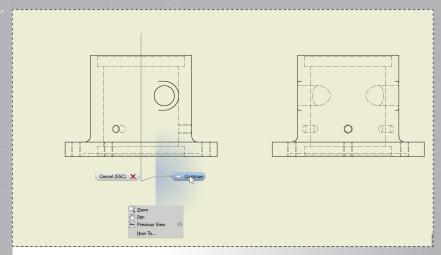
With the base view selected, open 'Section View' from the marking menu. Draw a vertical line through the middle of the part as shown. Right click and select 'Continue'.
