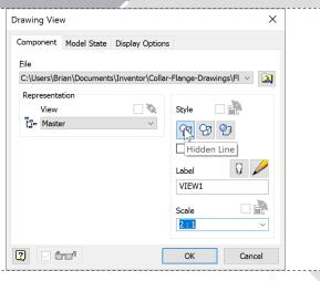
In the model window, right click to open the marking menu and choose 'Base View...'. Change the scale to '2:1' and ensure the style is set to 'Hidden Line' as shown.
