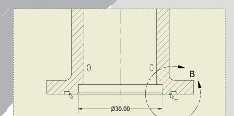
Select the two points shown to create an additional dimension. Place below the 30mm diameter dimension.
