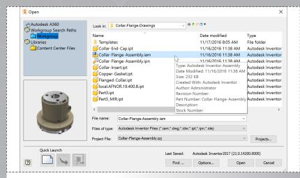
Start by clicking the 'Projects' icon in the ribbon. Navigate to where you saved the project files and select *Collar-Flange-Assembly.ipj*. Then open *Collar-Flange-Assembly.iam*.
