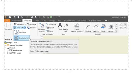
On the 'Annotate' tab in the ribbon, select the drop down arrow next to 'Ordinate' and start the 'Ordinate Set' command.
