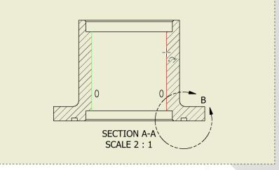
Select the edges as highlighted (green and red) to create a centerline in 'Section A-A'. Repeat to add centerlines in the Base and Right views of the part.
