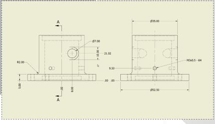
For additional practice, you can fully detail the Base and Right views as shown above using the techniques previously used. Save and close the drawing when complete.
