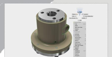
Select the *Flanged-Collar* component in the model window and right click to bring up the marking menu. Select 'open'.
