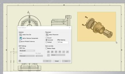
Click on the exploded view to 'Select View Set' and then window select all the parts for 'Add or Remove Components'.
