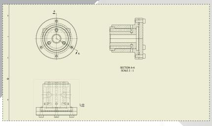
Repeat the 'Automated Centerlines' operation with the same settings in both the Top and Front views of the drawing.
