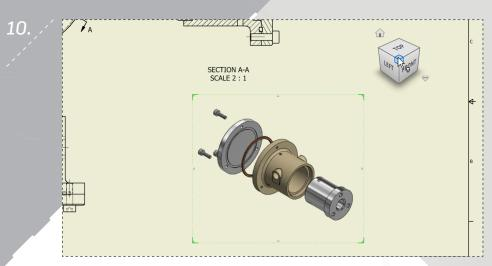
Click the corner of the ViewCube as shown to change to an isometric view of the exploded assembly. Move the view to the top right corner of the sheet.
