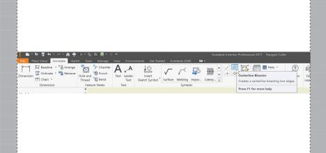
Using the same drawing created in Part 1, select 'Centerline Bisector' from the 'Annotate' tab in the ribbon.
