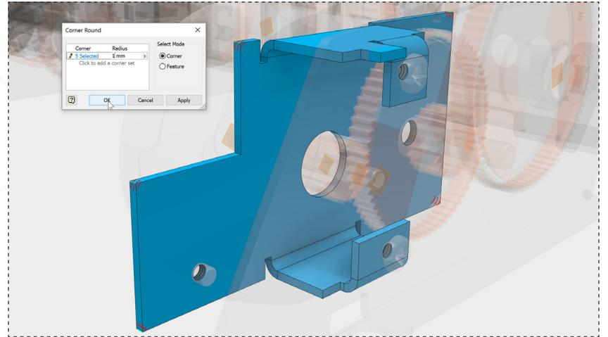
Select the edges as shown above and change the radius to 1mm. Click 'OK'. In the ribbon, select 'Return' to finish editing and save and close the files.
