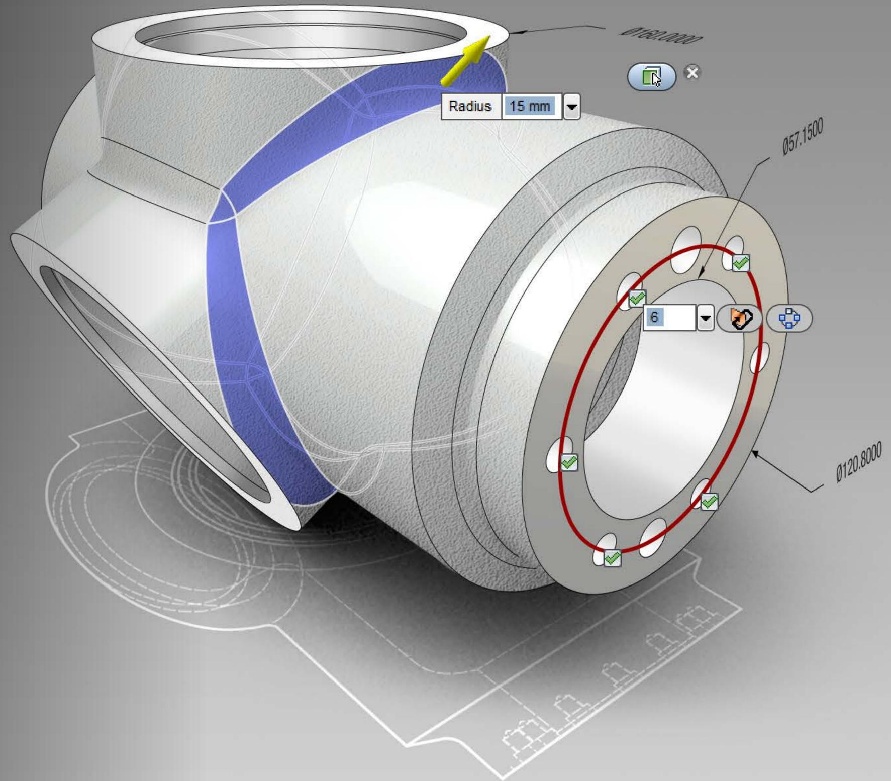
Parametric modeling is an approach to 3D CAD in which a model is built up step-by-step using features and constraints to capture design intent. Unlike direct modeling, designers can create parameters to sketch and dynamically size 3D objects.
