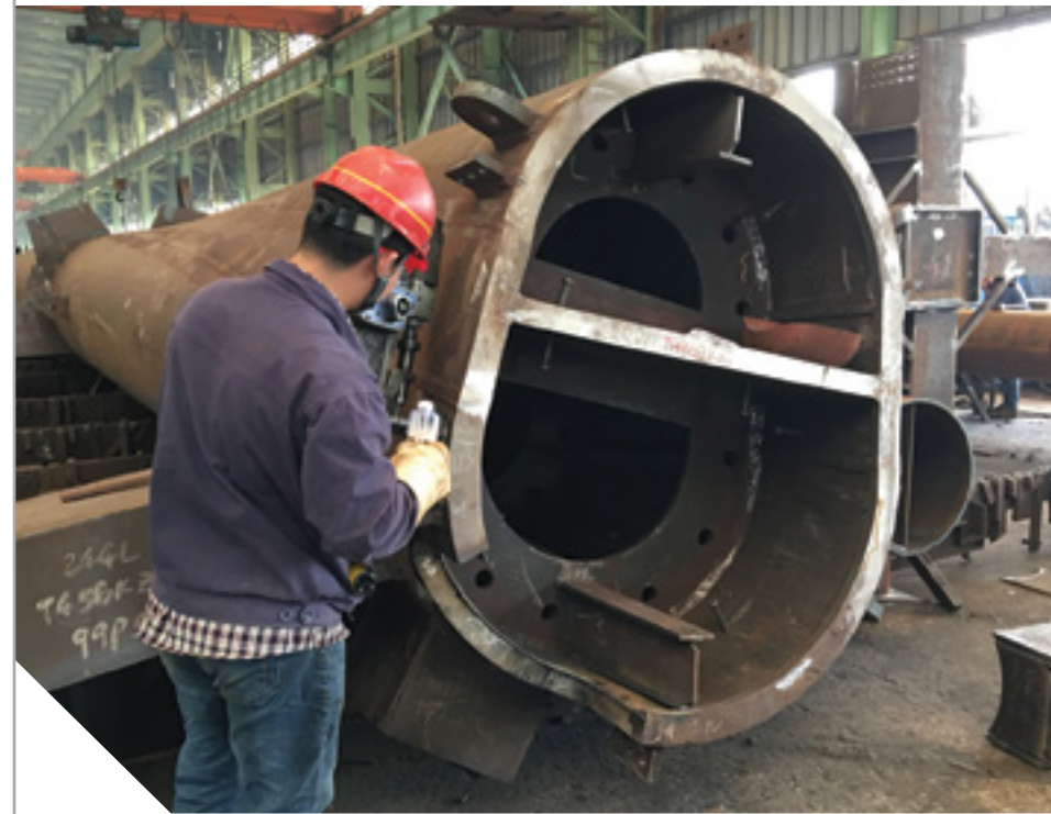
The tower's huge curved structural columns were manufactured off-site and assembled at the construction site. Courtesy China Construction Eighth Engineering Division.
