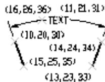
The point (15,25,35) specifies the vertex of the angle. The points (13,23,33) and (14,24,34) specify the endpoints of the extension lines. The point
