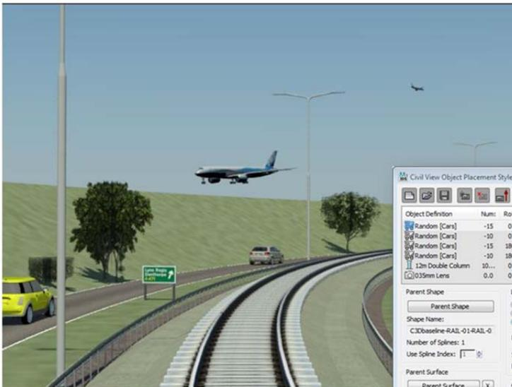
Figure 17. Civil View vehicle, lamp, tree, and sign objects placed in the scene using the Civil View Object Placement Style editor.
