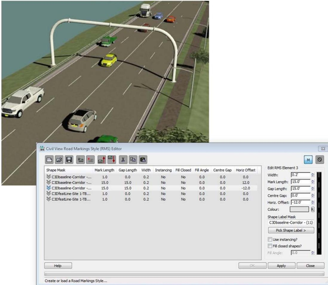
Figure 12. Civil View road markings and the Road Markings Style Editor panel.
