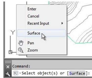
*Figure 32. Hide boundaries may now be added directly from other surfaces. For example, a corridor surface may be selected to create cutouts on an existing ground surface.*
