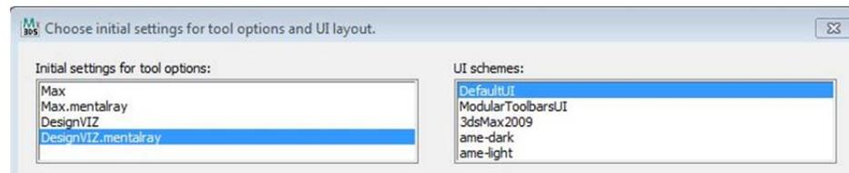
Figure 19. The initial settings for tool options and UI layout are set to give best results when using Civil View. These settings are accessed from the Custom UI & Defaults Switcher option in the Customize menu.
