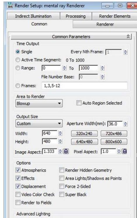
Figure 26. Rendering Parameters are set in the Common tab of the Render Setup panel.
