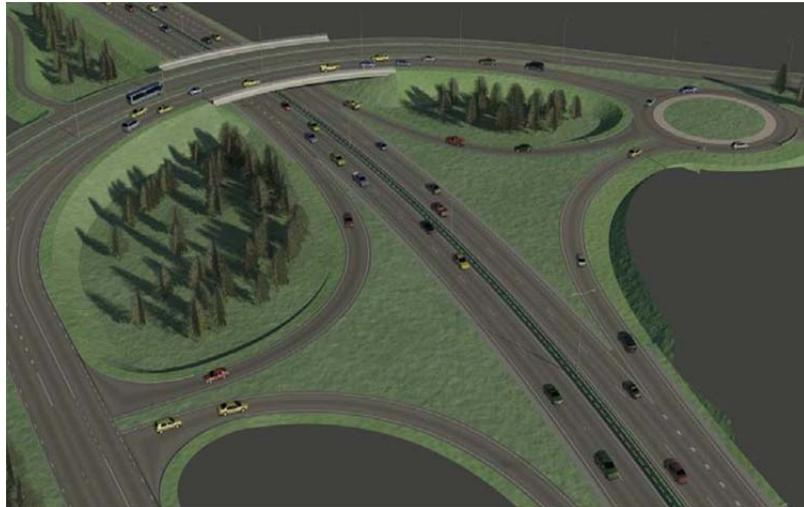
*Figure 3. Oranjewoud must verify the integrity of their AutoCAD Civil 3D design models, which makes design visualization an integral part of their design validation process.*
