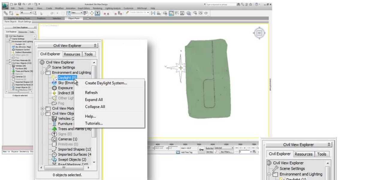
**Figure 21.** A daylight system is added to the Top view. Care must be taken when clicking and slightly dragging to place and size the compass icon, then a second click is needed to place the distant sun object icon.
