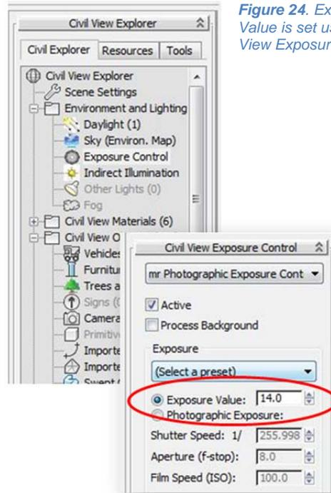
Figure 24. Exposure Value is set using Civil View Exposure Control.
