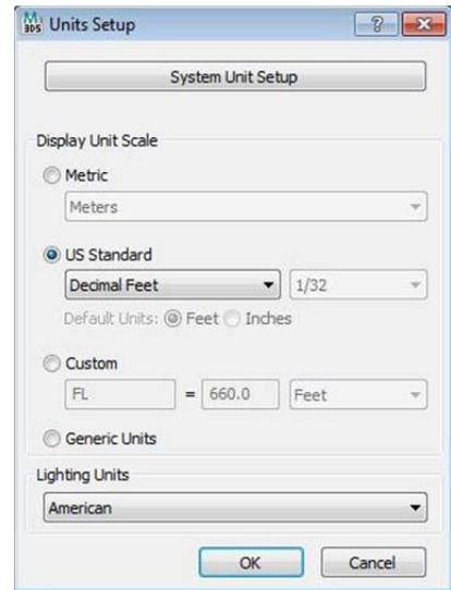
Figure 18. The 3ds Max Design units should be verified in the Units Setup panel.
