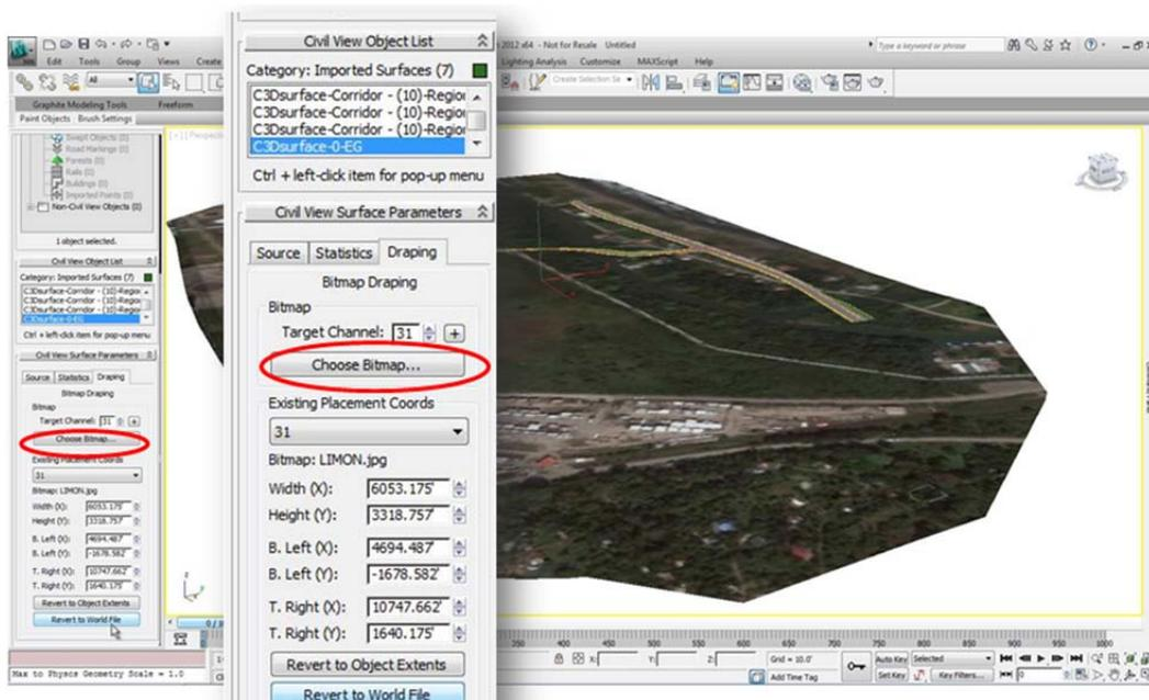
Figure 11. The imported surface before and after assigning and georeferencing the draped orthographic photograph.
