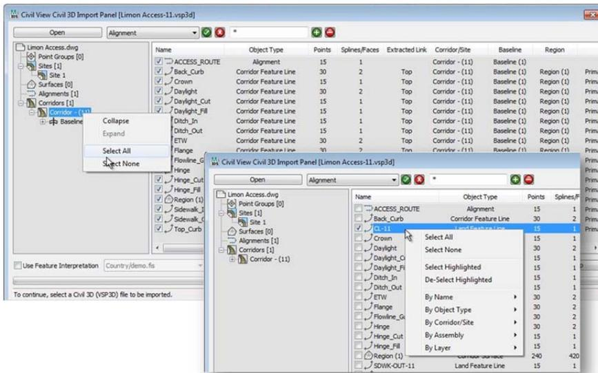
Figure 10. The Civil View import panel allows for group, individual, and filtered selection of model objects from the .vsp3d file to be imported into the Autodesk 3ds Max Design scene.
