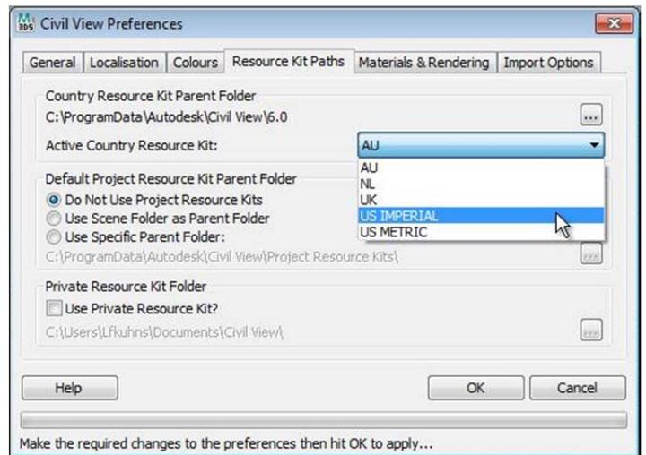
Figure 16. Country Resource Kits are used in Civil View to automatically apply localized standards to the objects placed in the scene. The active kit is selected on the Resource Kit Paths tab in the Civil View Preferences.
