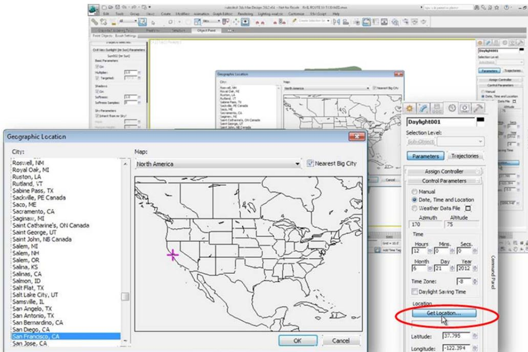
Figure 23. Parameters for the daylight system are set in the Motion area of the Command panel.
