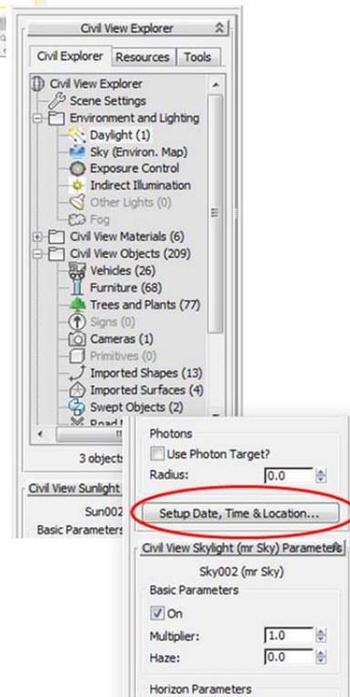
**Figure 22.** To set natural lighting parameters, select Daylight and then scroll down and select the Setup Date, Time, & Location button.
