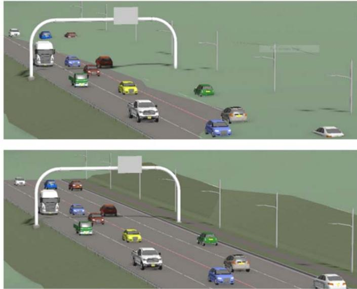
Figure 29. In the top image the existing surface has not been cut out and it obscures the design. In the bottom image a hide boundary created from the daylight limits of the design creates a cutout in the existing surface and the full design is displayed.
