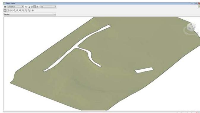
Figure 30. Objects are added as hide boundaries to the existing surface to create cutouts so the finished design data is not occluded.
