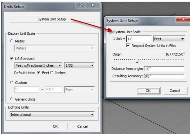
Figure 35. The System Setup dialog box.
