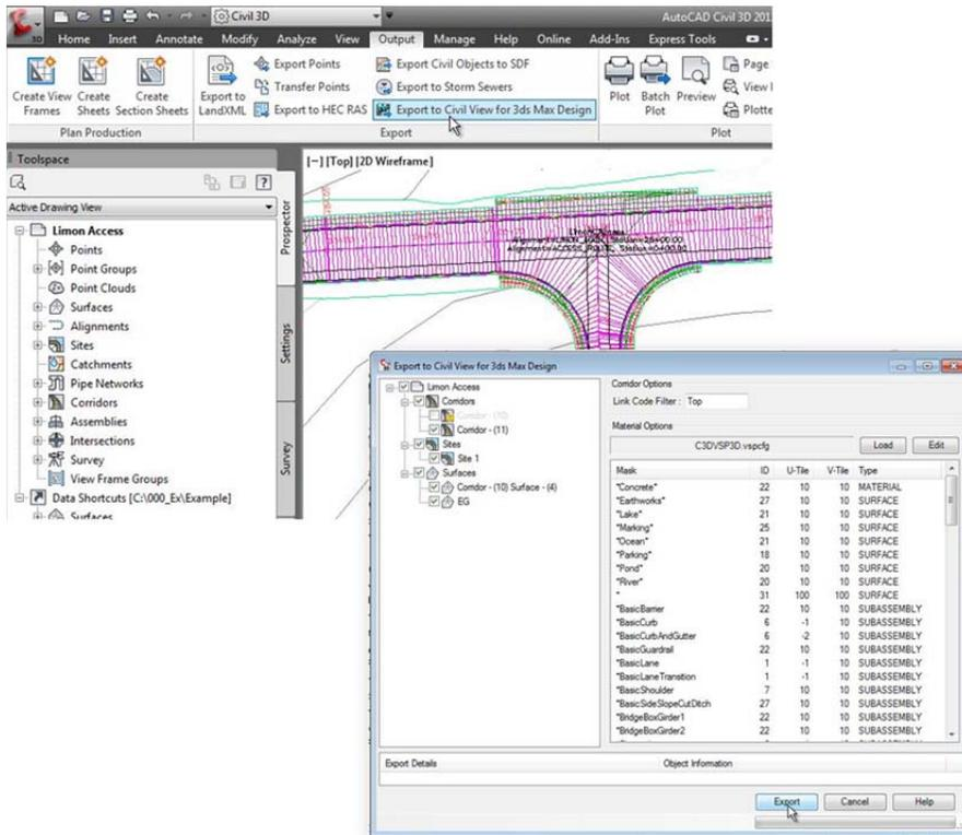
*Figure 8. Civil 3D model objects are exported to Civil View for 3ds Max Design from the option found in the Export panel of the Output display. The export creates a .vsp3d file type from the selected model objects.*
