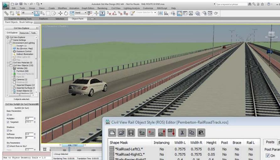
Figure 14. Civil View rail objects—both guardrail objects and railroad track objects—and the Rail Objects Style Editor panel.
