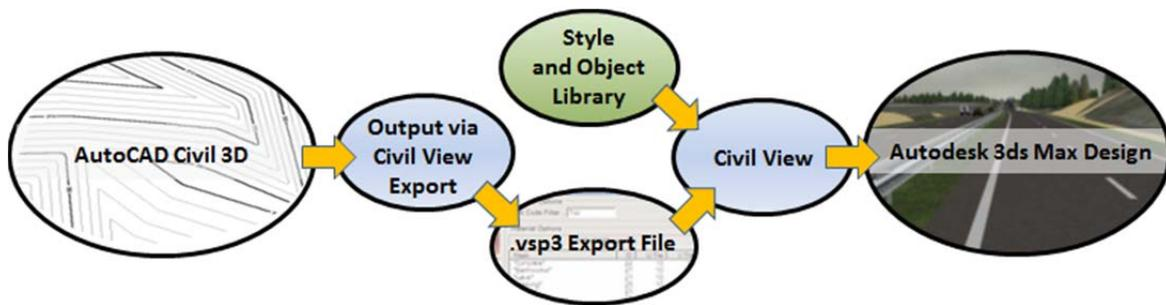
*Figure 5. The flow of civil design data from AutoCAD Civil 3D to Autodesk 3D Max Design using Autodesk Civil View for 3ds Max Design.*
