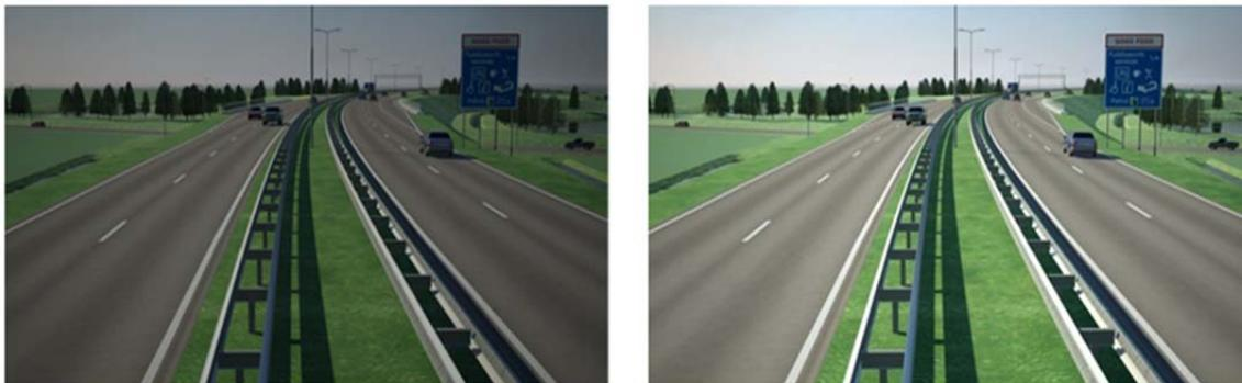
Figure 25. Exposure Values are needed to adjust output lighting levels. The higher the EV value the darker the scene. The scene on the left has an EV of 15; the scene on the right has an EV of 14.
