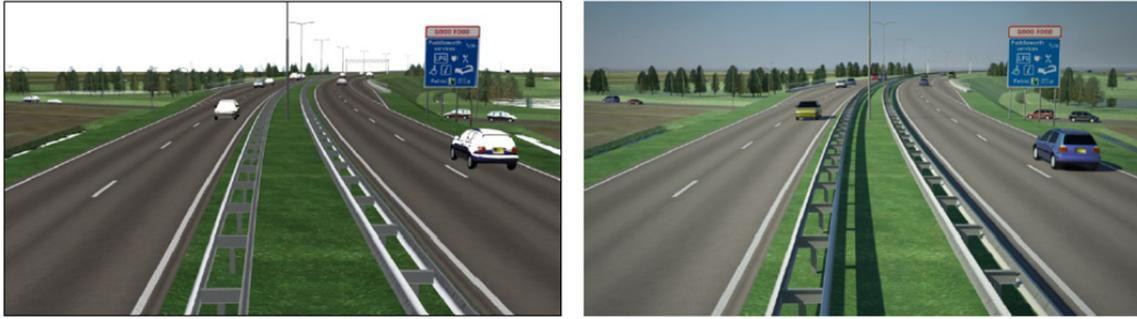
**Figure 20.** A comparison of before (left) and after (right) adding a mental ray daylight system to a scene. Note that using a daylight system provides the inclusion of shadows, which adds a sense of three-dimensional depth to the resulting image.
