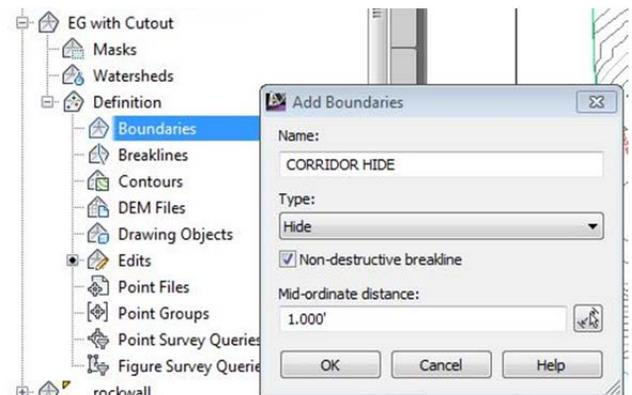
Figure 31. Hide boundaries are added to a surface definition to create cutouts.
