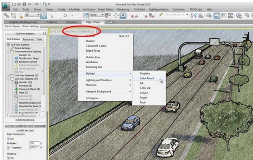
Figure 27. Scenes may be conceptually stylized using the Viewport Controls, and a still image can be saved by using the Grab Viewport command in the Tools menu.
