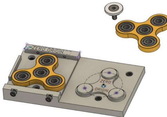
11. Once the joint relationship is complete, you will see that the four bearing components then move to be in the proper position as they belong to the rigid group relationship defined earlier within the Haas Fidget Spinner component document.
