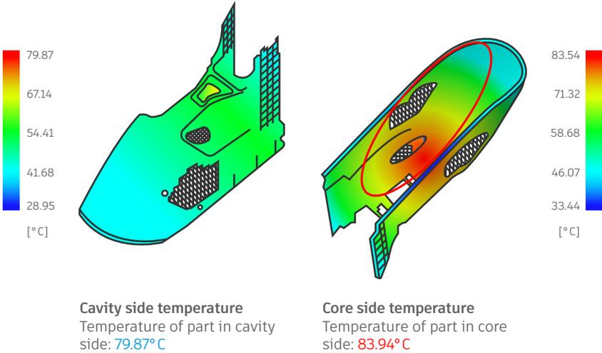
Figure 2: The warpage of the AC cover was caused by a temperature differential between the core and cavity side of the mold, as shown here.
