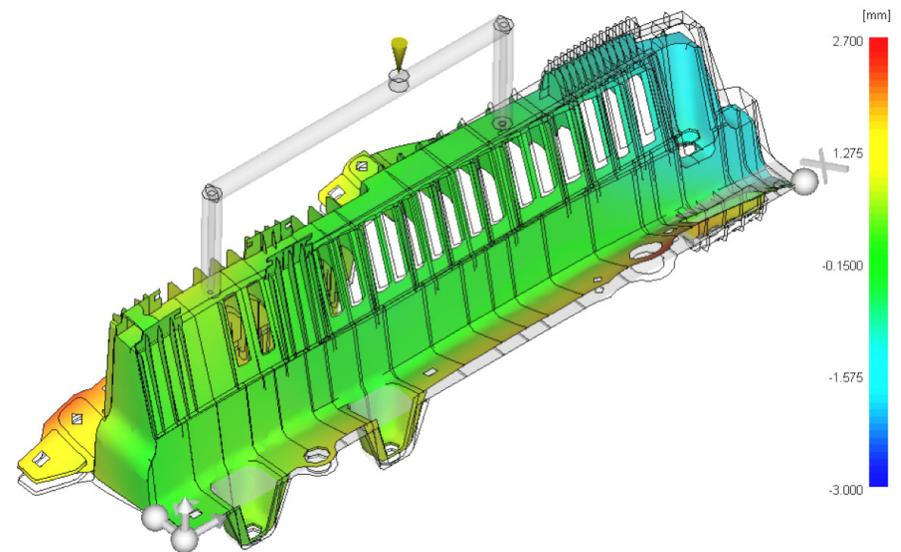
Figure 3: Using a DOE to eliminate options to change the process helped the engineering team quickly discover the use of sequencing valve gate openings to reduce the curvature of the upper surface of the part.
