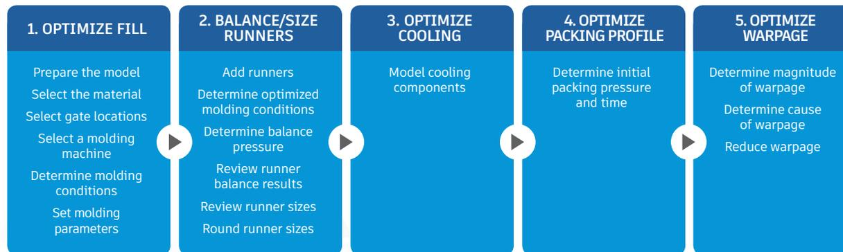
Figure 1: Because it depends so heavily on many other factors, optimizing warpage should be performed last after other steps have been perfected.
