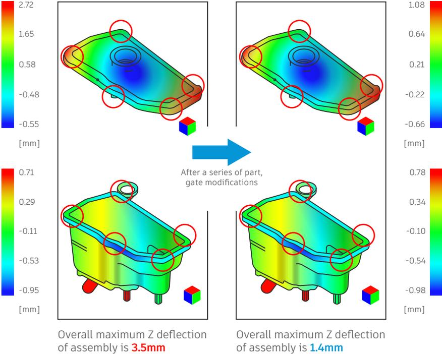
Figure 4: Parametric optimization allowed the team to evaluate 15 separate gate locations to identify the best solution.
