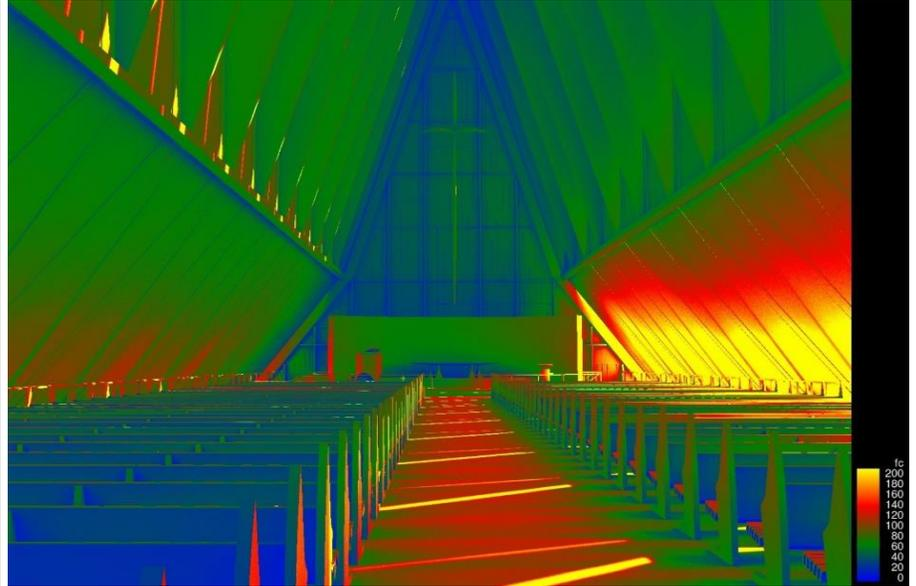
BIM-integrated whole building energy and daylighting analysis allowed the team to understand potential performance.
