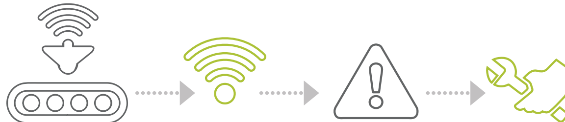
A conveyor belt with a noise sensor to detect shrieking when a belt is about to fail alerts the manufacturer of the typical lifespan of these components and identify points-of-failure that can be improved.
