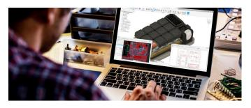
Fusion integrates mechanical CAD and electronics design, with schematic capture and PCB layout built into the workflow. Mechanical and electronic engineers collaborate in one environment for proper component alignment before manufacturing.
