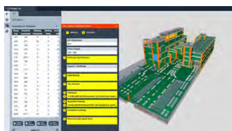
openBIM Model Checker automatically detects missing attributes Image Courtesy of CLP Power Hong Kong Limited
