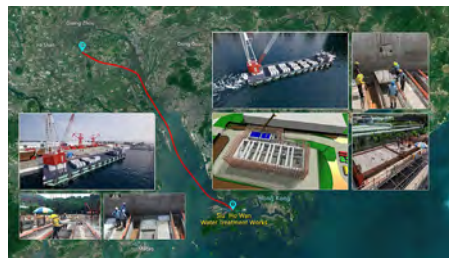
DfMA & MiMEP Transportation and Installation
