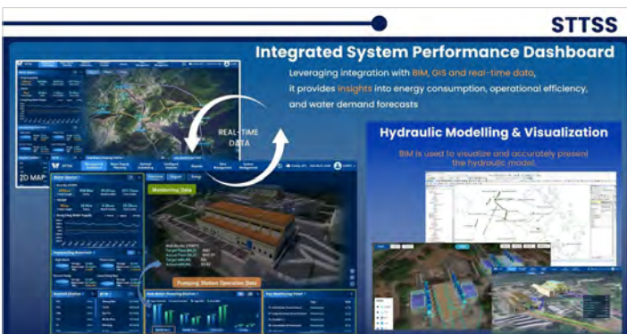
Image Courtesy of Water Supplies Department, HKSAR Government and Shenzhen Yuegang Technology Company Limited and The University of Hong Kong (HKU Business School) Utilizing BIM and GIS for Hydraulic Visualization of Dongjiang Water Mains in STSS
