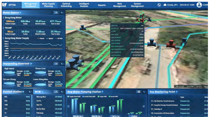
Image Courtesy of Water Supplies Department, HKSAR Government and Shenzhen Yuegang Technology Company Limited and The University of Hong Kong (HKU Business School) Real-Time Monitoring of Dongjiang Water Mains at STSS
