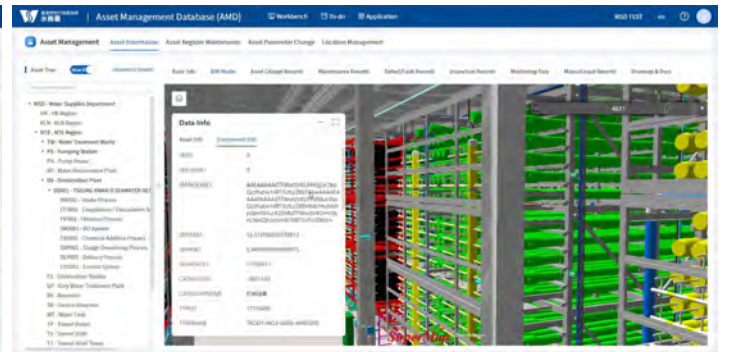
Utilizing BIM in AMIS for Asset Management Image Courtesy of Water Supplies Department, HKSAR Government and Shenzhen Yuegang Technology Company Limited and ACCIONA
