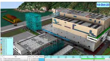
4D Simulation for MiC unit Delivery Image Courtesy of Environmental Protection Department, HKSAR and China Harbour Engineering Company Limited and Keppel Seghers – Zhen Hua Joint Venture
