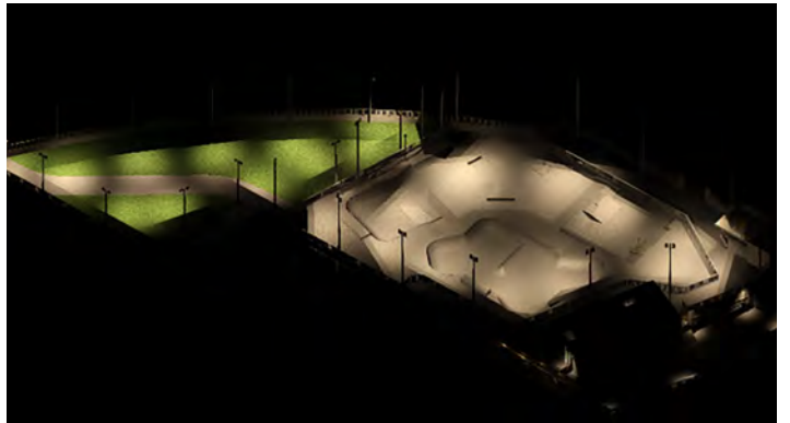
Skateboard Park Lighting Simulation and Lux Analysis through BIM Image Courtesy of Civil Engineering and Development Department, The Government of the Hong Kong Special Administrative Region and AECOM Asia Company Limited and DCKJV and TYFRON Consultancy Limited
