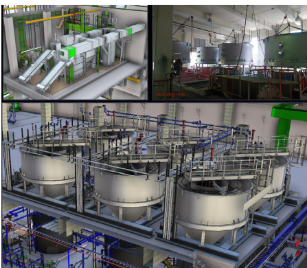
MIMEP of Lime Saturator and Lime Dross Recovery Tank
