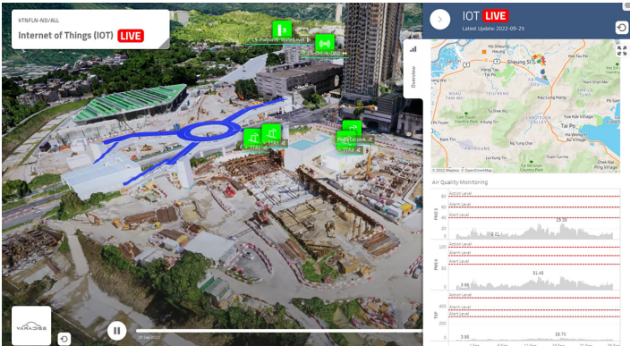
Central Management Platform Integration BIM with IoT for Real-time Site Monitoring Image Courtesy of Civil Engineering and Development Department, The Government of the Hong Kong Special Administrative Region and AECOM Asia Company Limited and DCKJV and TYFRON Consultancy Limited
