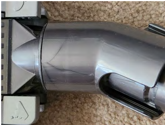
Figure 1. Molded vacuum swivel coupling and observed dark-line location.
