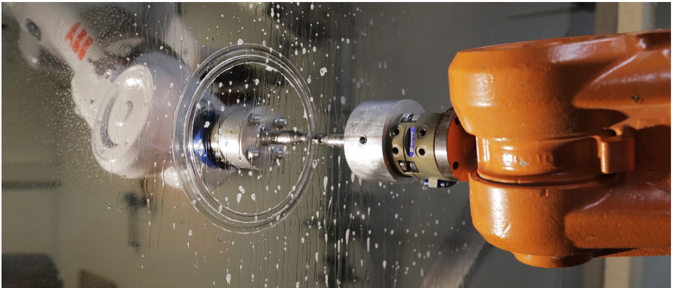
Incremental Sheet metal forming at CITA using two synchronized robotic arms
