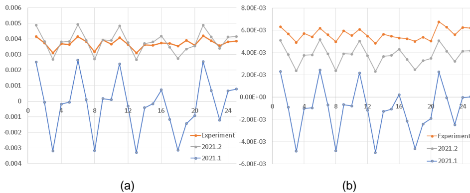
Figure 3: Shrinkage comparison for a 31% talc filled PP material in (a) flow direction and (b) transverse to flow direction.
