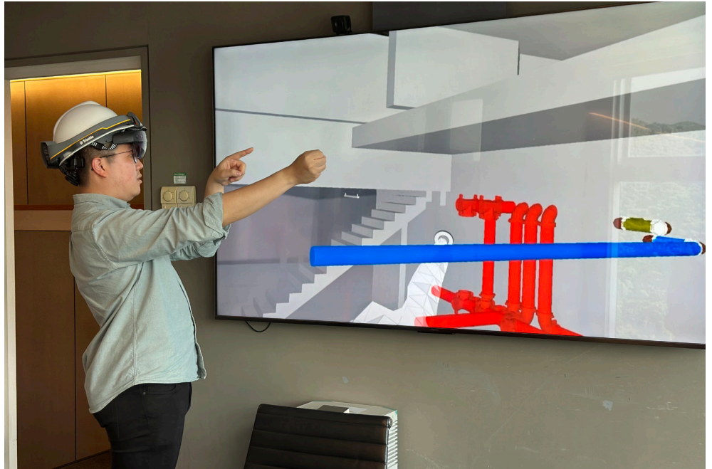
Mixed Reality airtightness review using HoloLens. Image Courtesy of Architectural Services Department, the Government of the Hong Kong Special Administrative Region and P&T Architects Limited and China State Construction Engineering (Hong Kong) Limited
