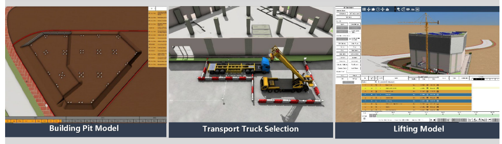
4D Phase Planning and Method Statement Simulation Image Courtesy of CRBC-QH-REC-QTEC Joint Venture and Binnies Hong Kong Limited and Huadong Engineering (Shenzhen) Corporation Limited
