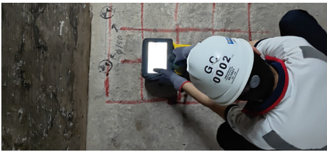
Concrete Scan Image Courtesy Hongkong Land Limited and Gammon Construction Limited
