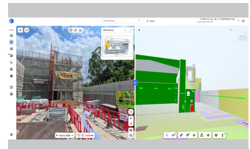
AR/MR is used to overlay BIM models for real-time site inspection and collaboration Image Courtesy of CLP Power Hong Kong Limited and Hip Hing Construction Company Limited and Andrew Lee King Fun & Associates Architects Limited
