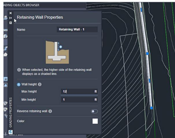
The Feature Line Edit tools are a key to proper creation of a retaining wall in the standard grading tools in Civil 3D.
