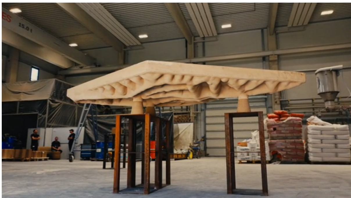
Figure 8. Completed 4 meter span prototype floor slab. The stay-in-place, 3D-printed formwork and the continuous flax-fibre winding now act as a single, integrated load-bearing system.
