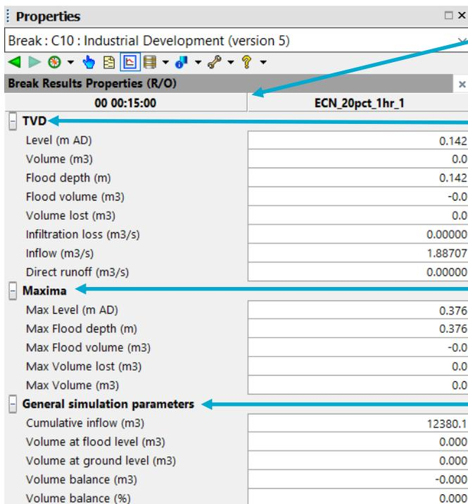
**Time and simulation:** this states the timestep of the results and the simulation name.
