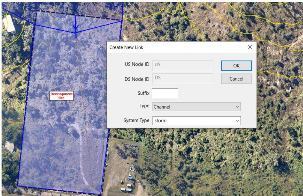
10. The properties page for the new channel should appear and ICM will provide a red validation error where the invert levels and section shape need to be populated. Set the **US invert** to **20** and **DS invert** to **10**.
