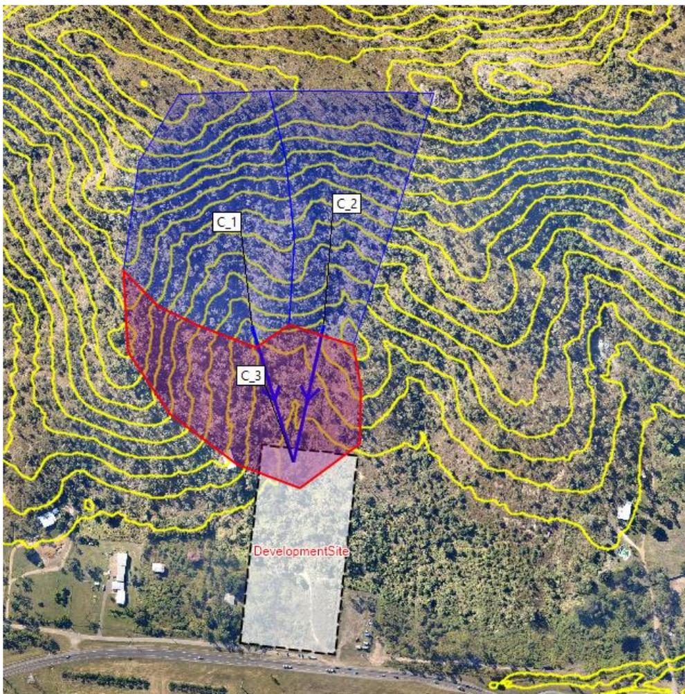
4. Lastly, set the **Output lag (minutes)** to **5** and check on the **Bypass runoff** for both subcatchment **C\_1** and **C\_2**. This can be done in the property window for each subcatchment or in the subcatchment grid windows.
