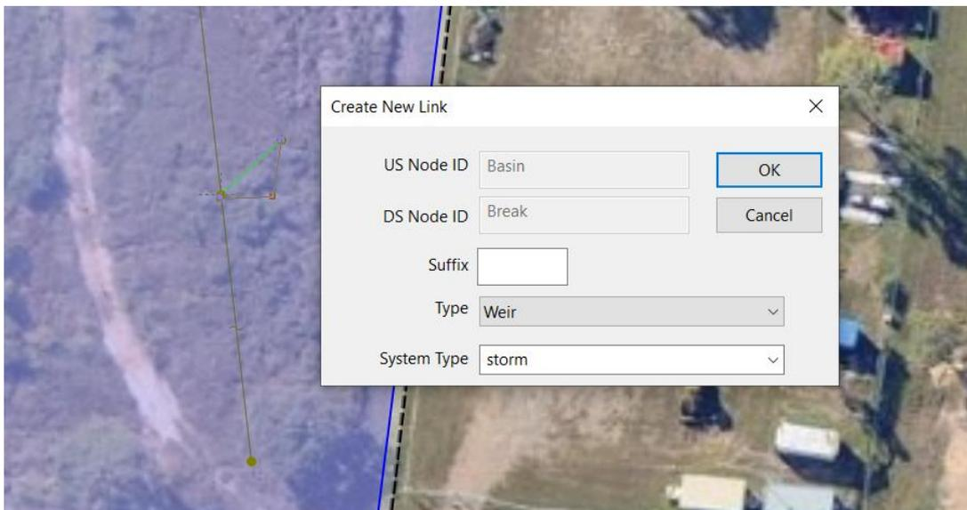
8. In the properties dialog, set the Crest (m AD) to **12.8** (0.8m above the storage invert), the Width (m) to **3** and the Discharge coefficient to **0.64**.
