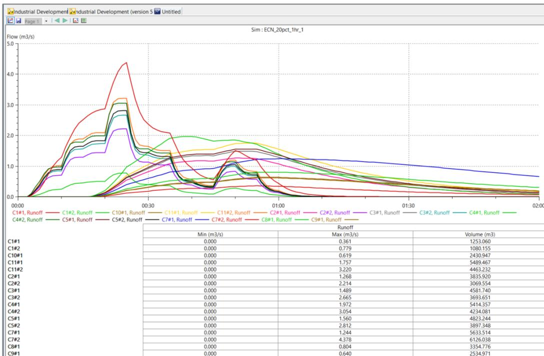
The result grids tabulate all the result information for the individual objects. You will see the default layout when we open the results grids. This can be customised and saved so that the most useful information is moved into the left-hand columns for easier viewing.
