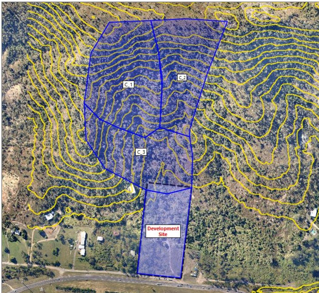
15. We can use the Model tools to ensure the 4 subcatchments have snapped vertices and no gaps or overlaps. Hold down CTRL to select all 4 polygons using the select tool. Alternatively, you can right-click on **Subcatchments** in the **Key** window and choose **Select objects**.
