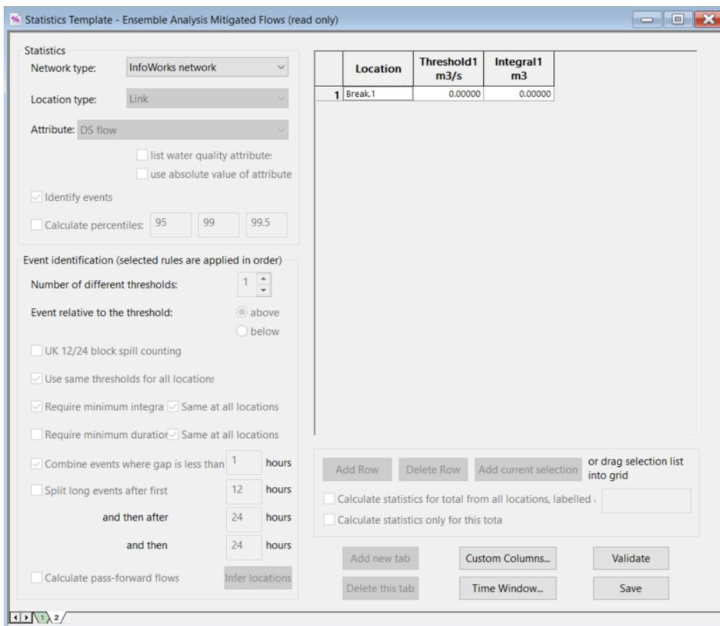
18. Go to **Results > Statistical reports...** and add the mitigated run results and the new statistical template. After producing the results from the dialog, you can add the box and whisker plot by going to **Statistics > Export box and whisker plot**.
