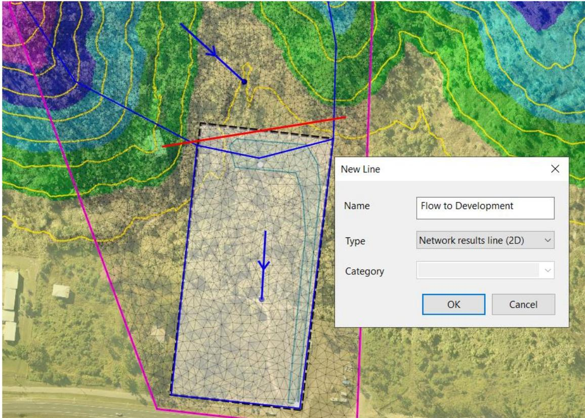
24. Re-mesh the 2D zone to incorporate the diversion channel and network result line.
