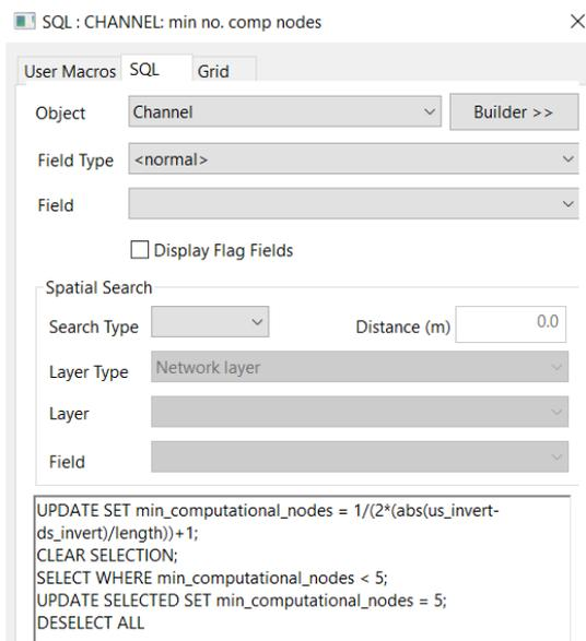
3. Drag the SQL onto the GeoPlan and open the properties for a few of the channels in the model. The min. computational nodes field will be updated from 5.
