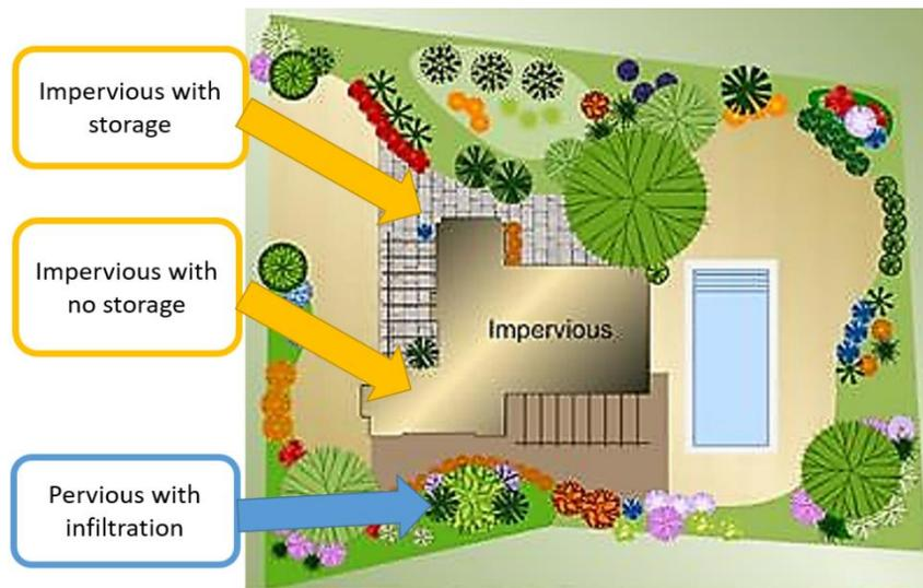
In the example above, we can assume that this typical **Urban Land Use** has 3 types of **Runoff Surfaces**: Impervious with Storage, Impervious with no storage, and Pervious with Infiltration. Each surface has its own characteristics, and runoff subcatchment when rainfall falls on them.
