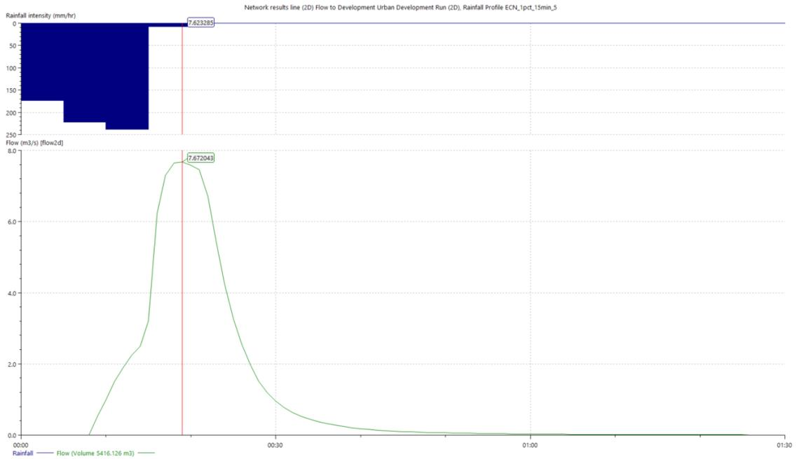
32. Compare the result with the same storm simulation completed in the **Urban Development (Pre-dev) Run**. Graph the **Total outflow (m<sup>3</sup>/s)** attribute for Subcatchment **C\_3**. The estimated peak flow is around 8.1 m<sup>3</sup>/s occurring 17mins after the beginning of the storm.
