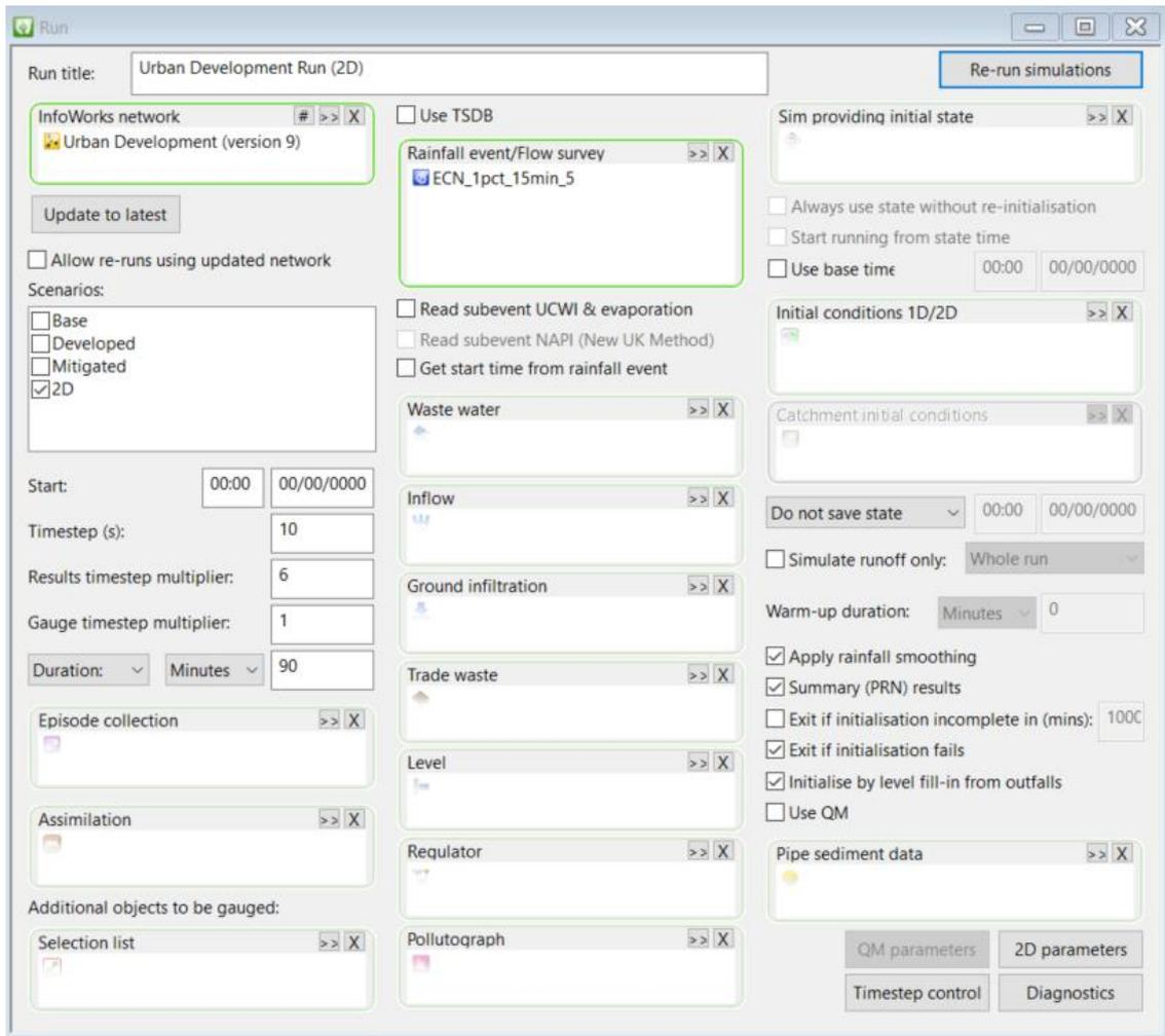
**NOTE:** 2D calculations can be accelerated significantly by accessing any available GPUs. To use a GPU card for the 2D calculations click on **2D Parameters** in the Run object window and navigate to the **GPU** tab. If 'Always' is selected and no GPU is present the run will fail.
