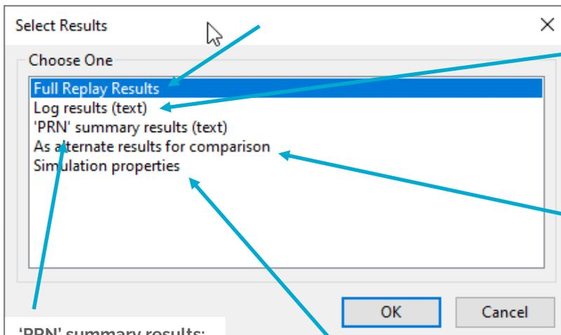
**Log results:** A breakdown of the simulation, any simulation errors are listed here; this is especially useful if the model is not completely successful.
