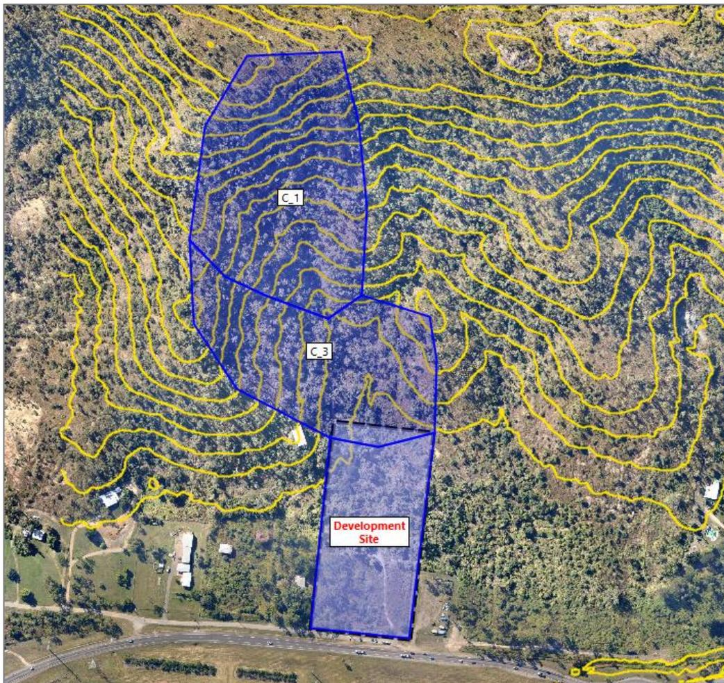
**Note** that the subcatchments do not cover the full area draining to the top of the development site. We will add the missing Subcatchment manually using the Geoplan tools.
