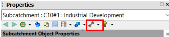
18. Right click within the Object properties window and select **Add group**. Call the new group **RAFTS**. Ensure that the new RAFTS group is moved to the top of the window.
