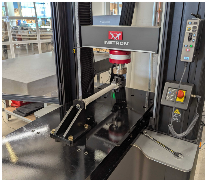
Figure 7: Instron sensor test rig loading setup
