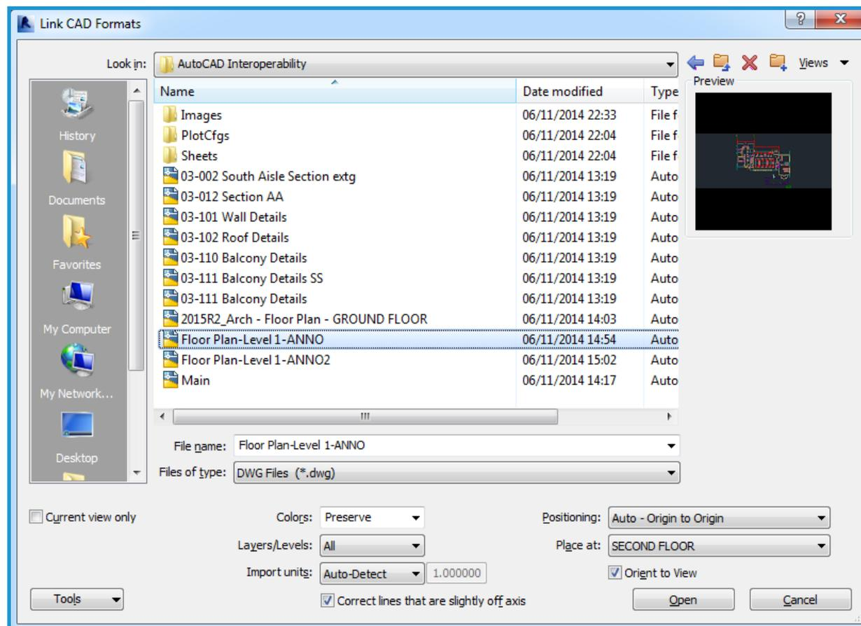
After the file is linked, suppress display of the Revit-generated elements. In AutoCAD, unload the Revit exported file. Return to Revit and click Manage Links from the File menu. Select the linked file, and click Reload.
