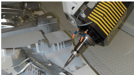
CNC machining of steel injection mould tool
